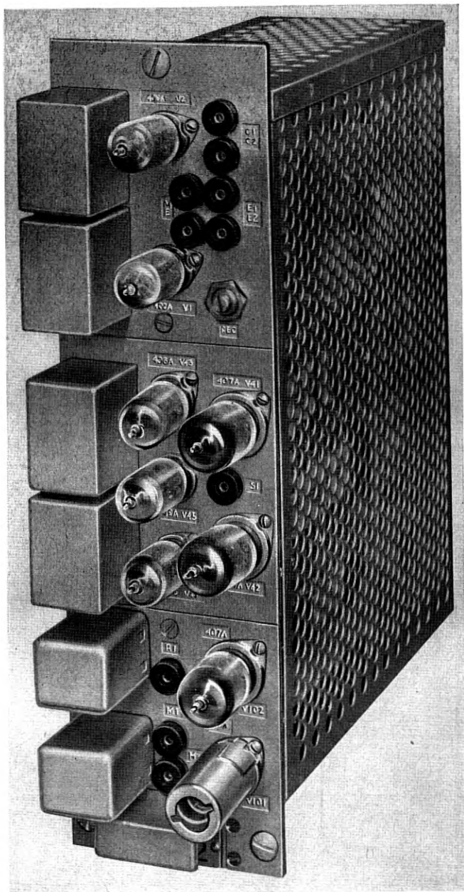
Fig. 16—Channel unit—front view. The unit is equipped with a perforated aluminum can cover.
