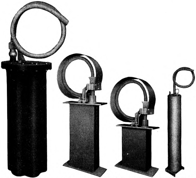
Fig. 18—Progressive case size reduction 1925–1942 200-coil complements—88 mh. loading coils. Left to right: No. 602 (hard iron-wire core) coils in cast iron case; No. 612 (permalloy core) coils in “thick” steel cases, welded joints; No. 622 (molybdenum-permalloy core) coils in “thick” steel cases; No. 632 (molybdenum-permalloy core) coils in tubular “thin” steel cases.
