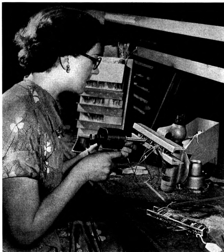
Fig. 12—Operator using electrically operated wire wrapping pistol. All wires are precut to suitable length.
