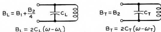
Fig. 4.15—The approximate variation with frequency (over a narrow band) of the longitudinal ( B_L ) transverse ( B_T ) susceptances of a filter network.
