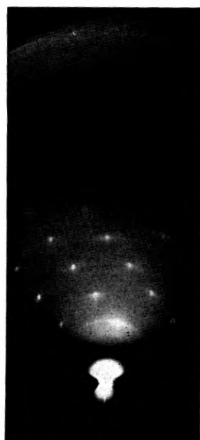
Fig. 13.—Electron diffraction photographs of a BT quartz plate taken with a 50 kv. electron beam (C. J. Davisson)
