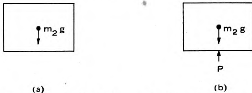
Fig. 1.2.2—Free body diagram for elementary system.
