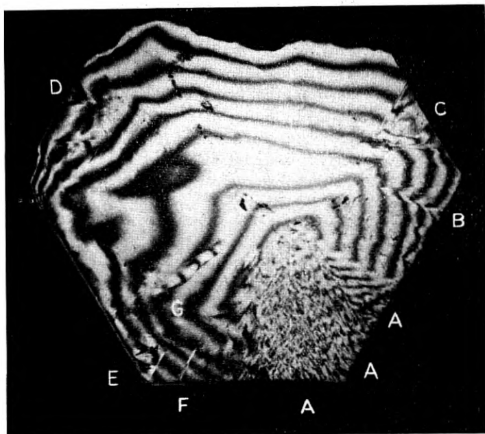
Fig. 4.8—A broken cap of quartz is viewed along the optic axis in polarized light. Few, broad thickness-contours show good alignment with the optic axis. The fine TOOTHED-PATTERNS are due to optical twinning.
