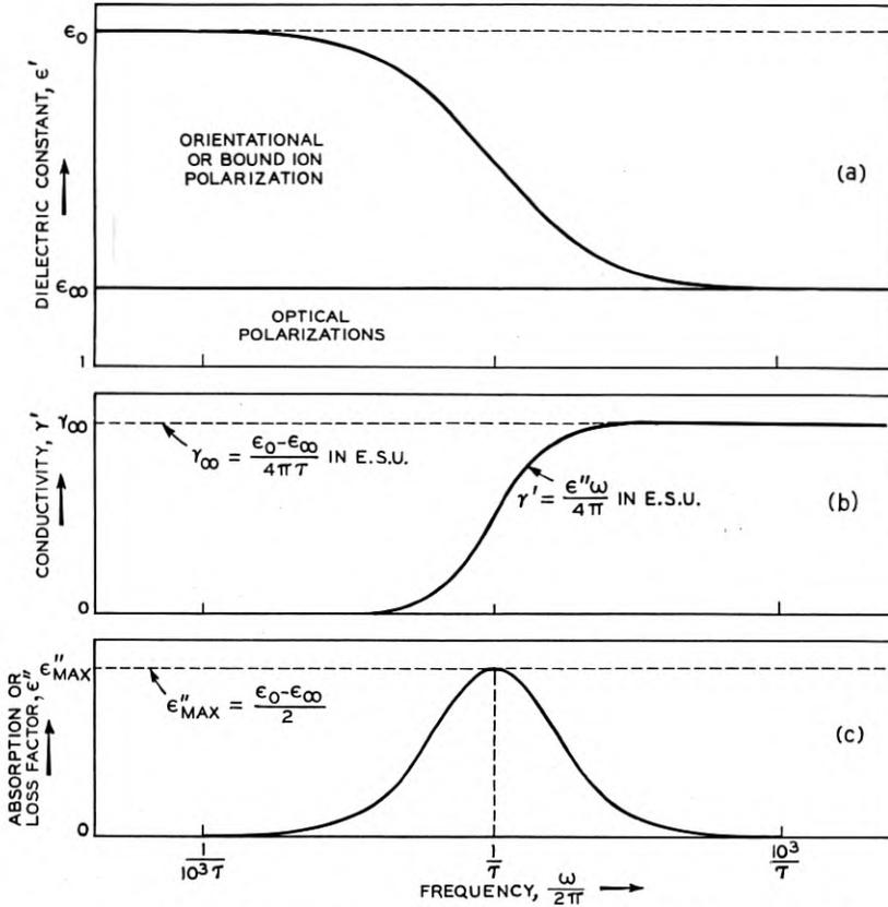
Fig. 1—Schematic diagram comparing the frequency dependence of dielectric constant ( $\epsilon'$ ), loss factor ( $\epsilon''$ ) and conductivity ( $\gamma'$ ). This applies to a polarization having a single relaxation-time ( $\tau$ ). The frequency in cycles per second is  $\omega/2\pi$ .
