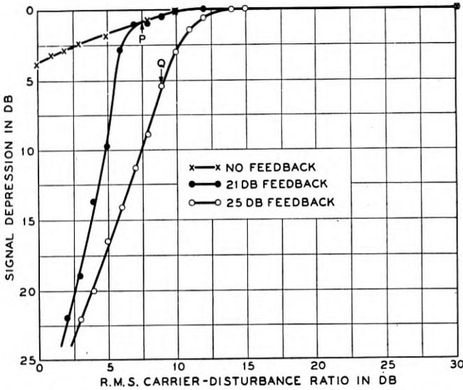
Fig. 14—Depression of output signal by the disturbance. Modulation:  $\pm 7$  kilocycles for no feedback,  $\pm 78.5$  kilocycles for 21-decibel feedback, and  $\pm 124.5$  kilocycles for 25-decibel feedback. Points *P* and *Q* denote incidence of cracking in the absence of modulation, for 21- and 25-decibel feedback, respectively.
