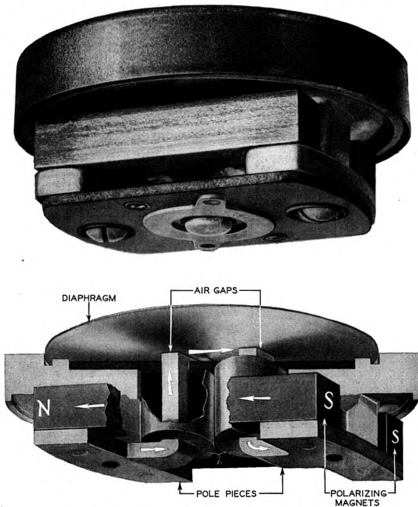
Fig. 6—Magnetic circuit of the new telephone receiver.
