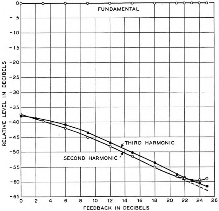
Fig. 9—Effect of feedback upon receiver distortion. Fundamental level kept constant by increasing transmitter modulation in proportion to the feedback. Modulation with no feedback =  $\pm 7$  kilocycles at 1000 cycles per second.
