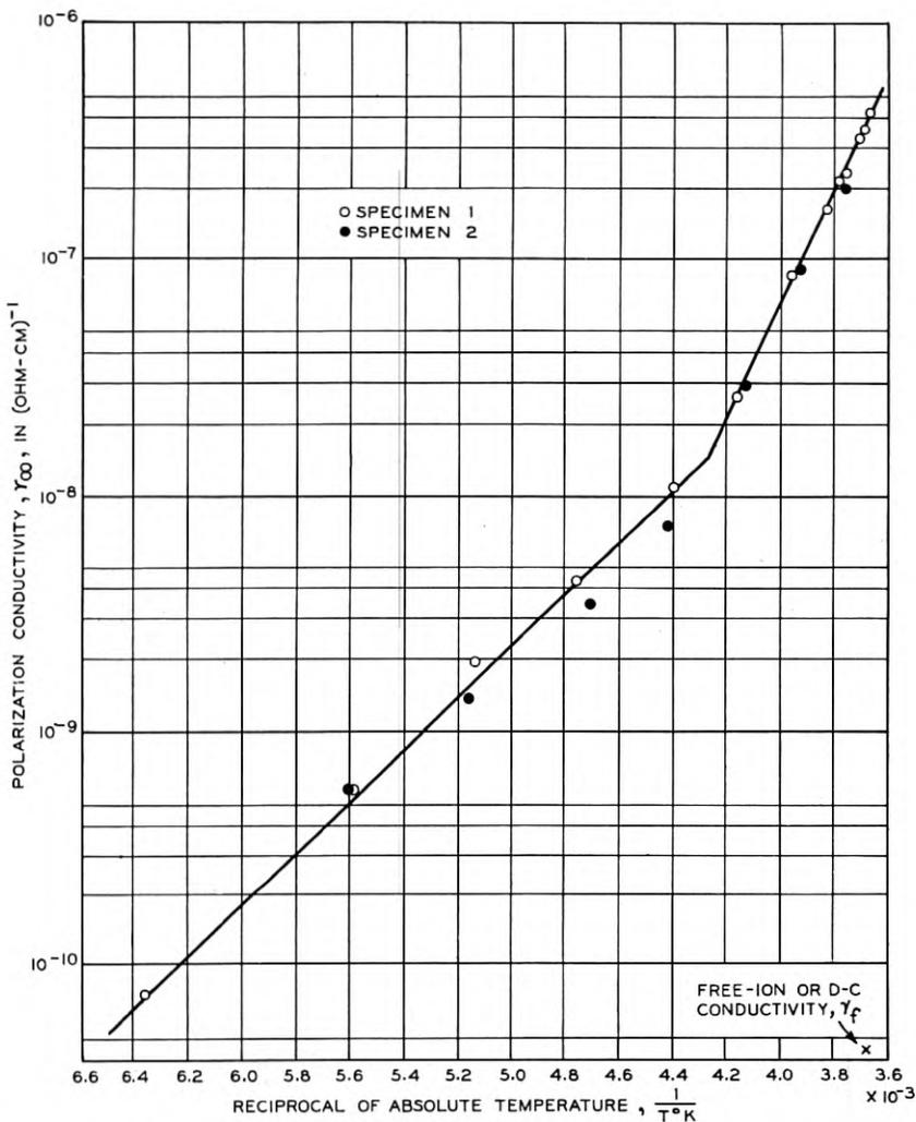
Fig. 5—An illustration of polarization conductivity. The temperature-dependence of the polarization conductivity of pure ice in the range  $-0.8^{\circ}\text{C}$  to  $-190^{\circ}\text{C}$ . The free-ion (or d-c) conductivity is also shown for a single temperature.
