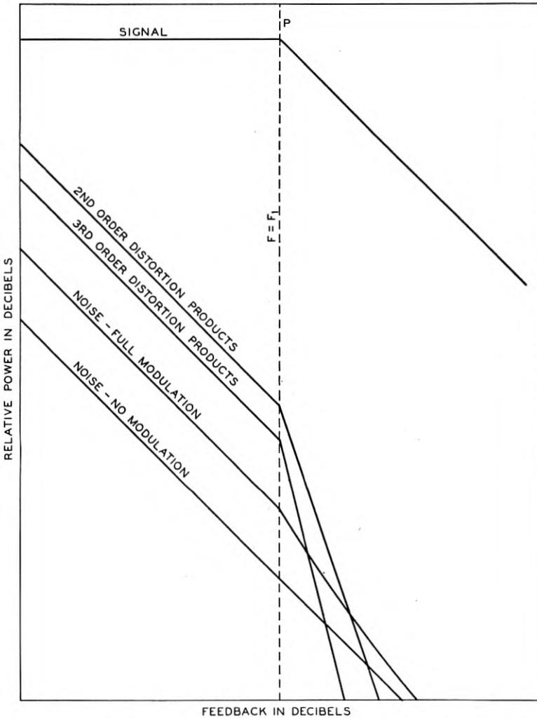
Fig. 3—Theoretical manner in which components of receiver output are modified by feedback. Modulation level at transmitter is assumed to be increased by the feedback factor up to point  $P$ , and subsequently to remain fixed.
