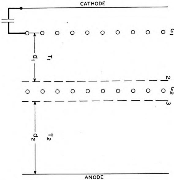
Fig. 3—Schematic of a space charge grid tube.
