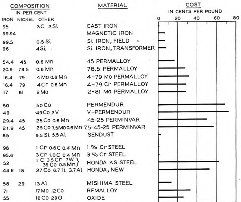
Fig. 3—Raw materials cost of various magnetic alloys.
