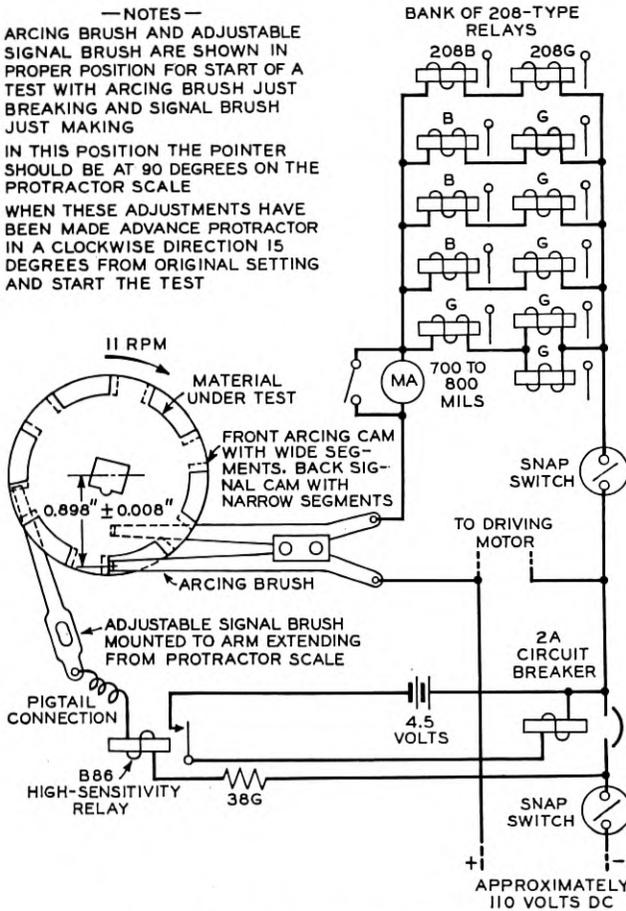
Fig. 8—Circuit for arc resistance test.
