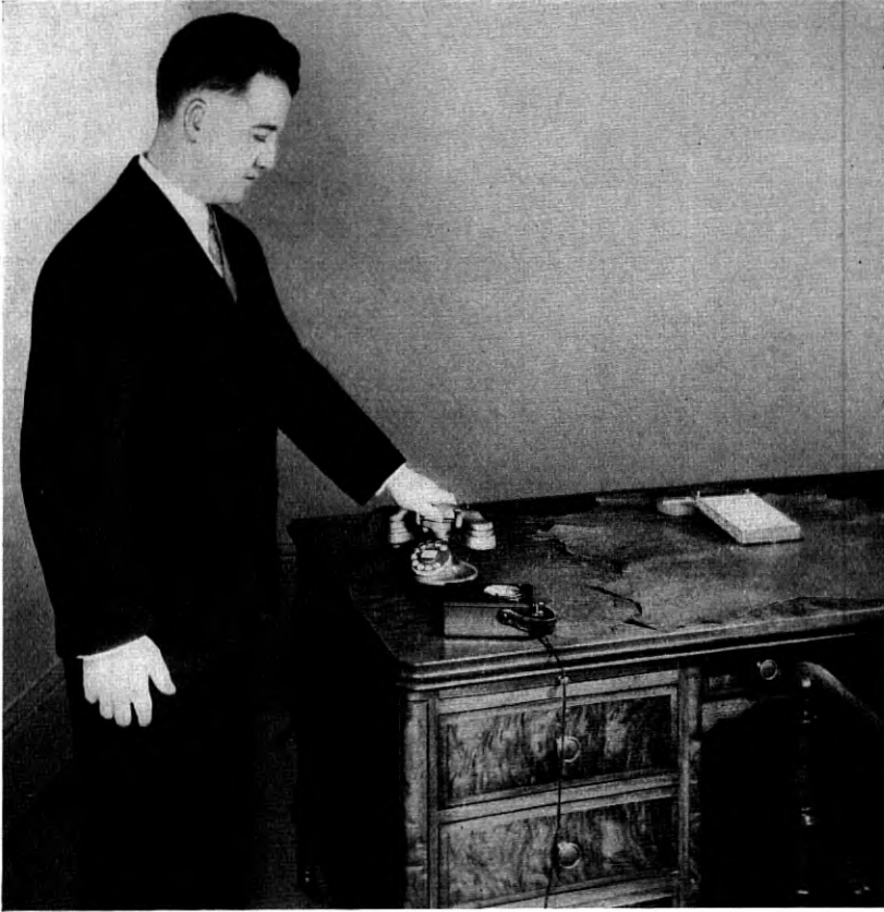
Fig. 6—Small receiving set as used to measure the transmission loss of a subscriber's line. The 1000-cycle generator has been connected to the central office end of the line by calling a designated number. When the telephone instrument has been replaced on the mounting, the meter in the measuring set will read the line loss.
