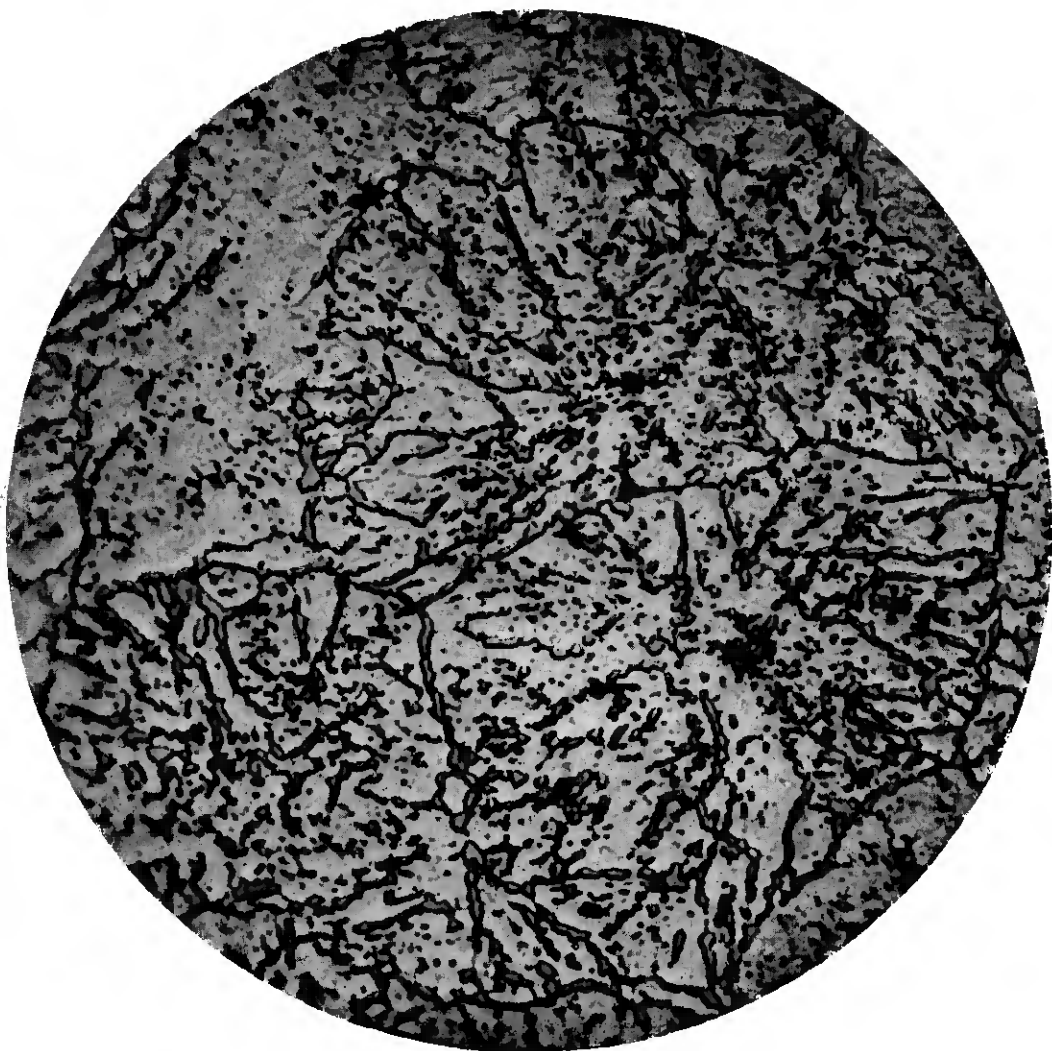
Fig. 14—Mag. 3500X. Fig. 14 is of a specimen which was quenched and then drawn for ten minutes at 650^{\circ}\text{C} . The outline of a troostitic nodule is clearly marked by globular carbide particles. The hardness of the specimen was C-28 after tempering.
