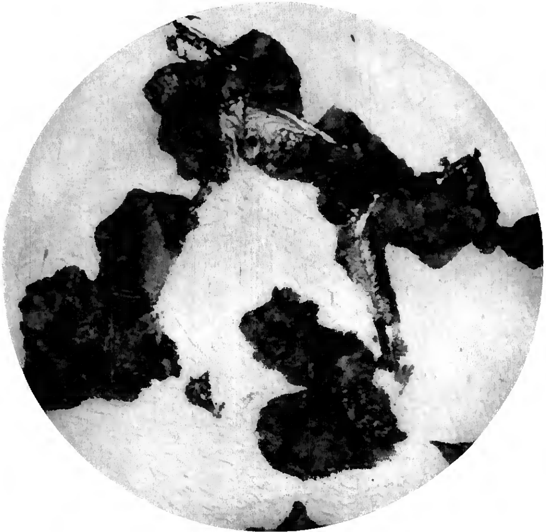
Fig. 4—Mag. 3500X. Fig. 4 shows a somewhat later period in development of troostite. The troostite appears to have formed along grain boundaries. The excess constituent is clearly seen, and here and there a laminated structure, pearlite. Evidently whatever the state of the carbide with reference to the iron in troostite—whether contained in solid solution as first formed or whether disposed as a fine aggregate with the iron—the condition must be very unstable, otherwise evidences of finely laminated pearlite would be lacking.
