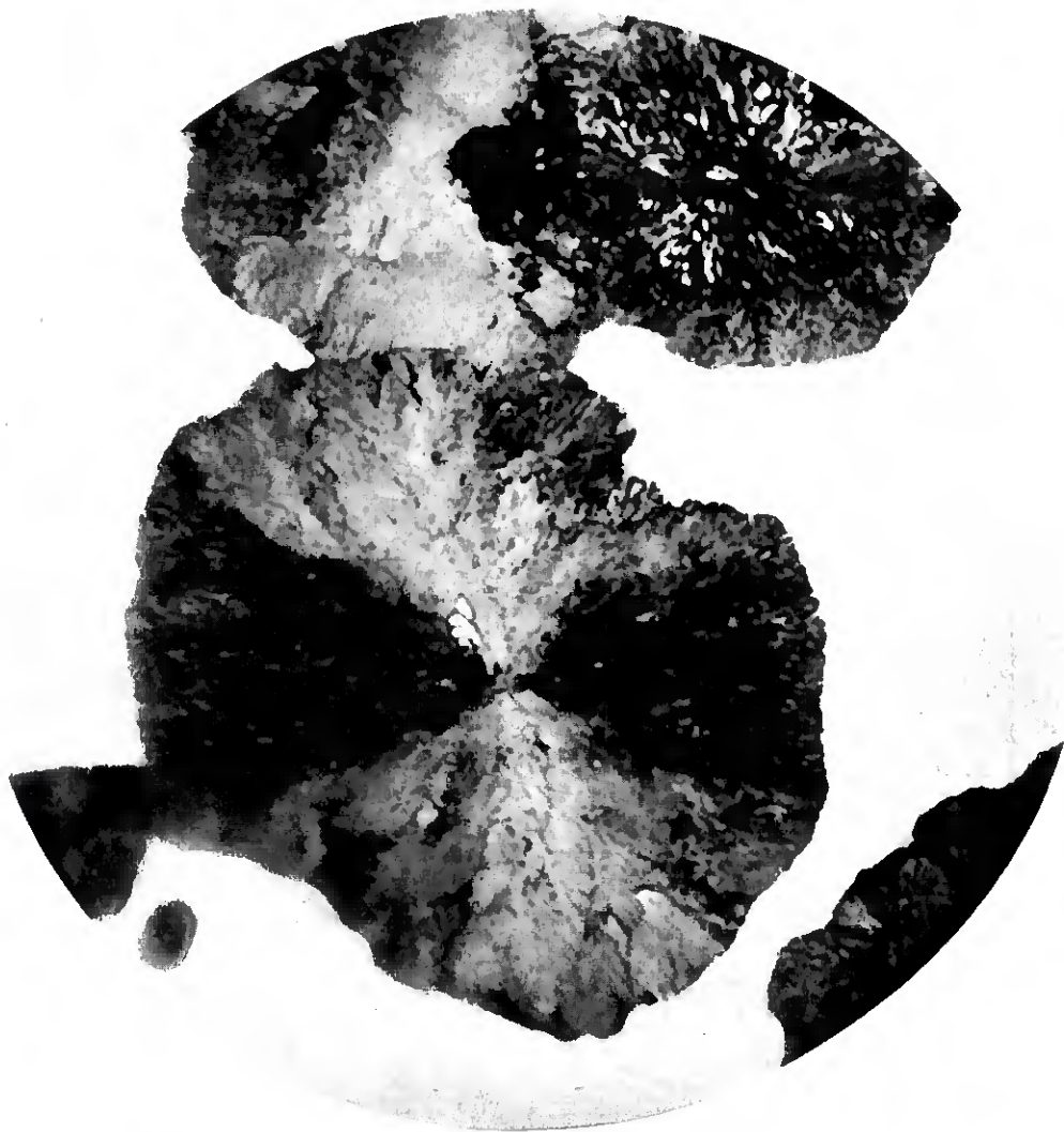
Fig. 5—Mag. 3500X. Fig. 5 is of a small but well developed nodule showing four fan-shaped grains about a nucleus of growth. Some excess constituent has appeared but only the very early stages in the process of stratification to pearlite are visible. It is apparent, however, that the nodule is not composed of a solid solution. The nodule is about eight ten-thousandths of an inch in diameter.
