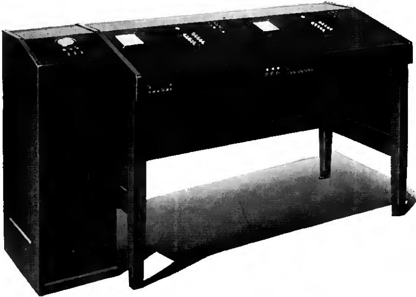
Fig. 31—Step-by-step dial tandem board. Calls completed to the terminating dial subscriber station by means of the 10 button key set shown on the keyboard. Incoming calls automatically distributed to an idle operator.
