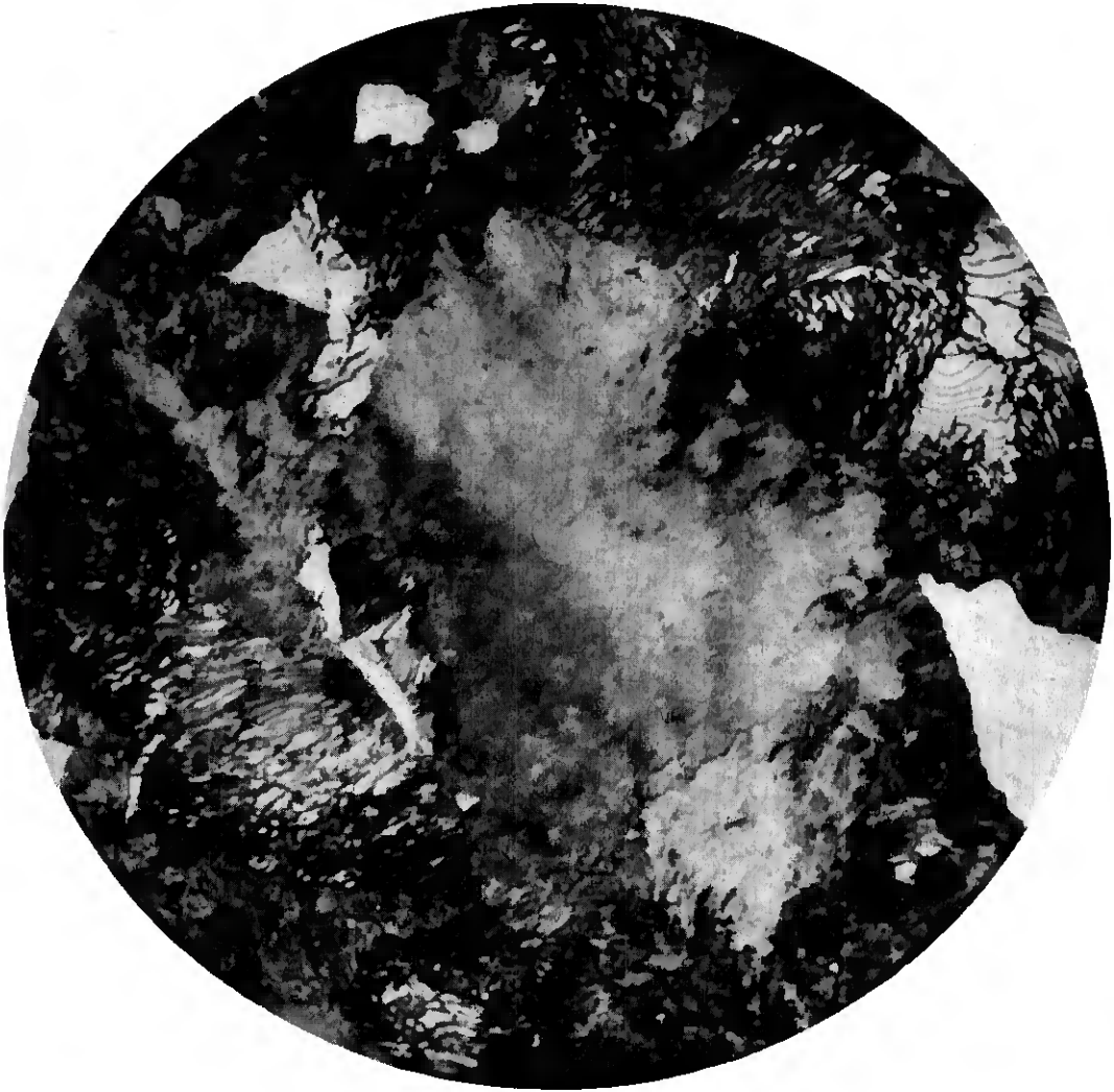
Fig. 8—Mag. 3500X. Fig. 8 shows a troostitic development which had formed along an old austenitic grain boundary. The excess constituent is starting to clear at the grain boundary. Well developed pearlite is revealed. The large light-colored grain covering the center of the field is just starting to break up into two constituents. Formerly grains of this kind, because of lack of resolution, were thought to be in all probability solid solution grains. These grains must represent a state very nearly that of freshly formed troostite.
