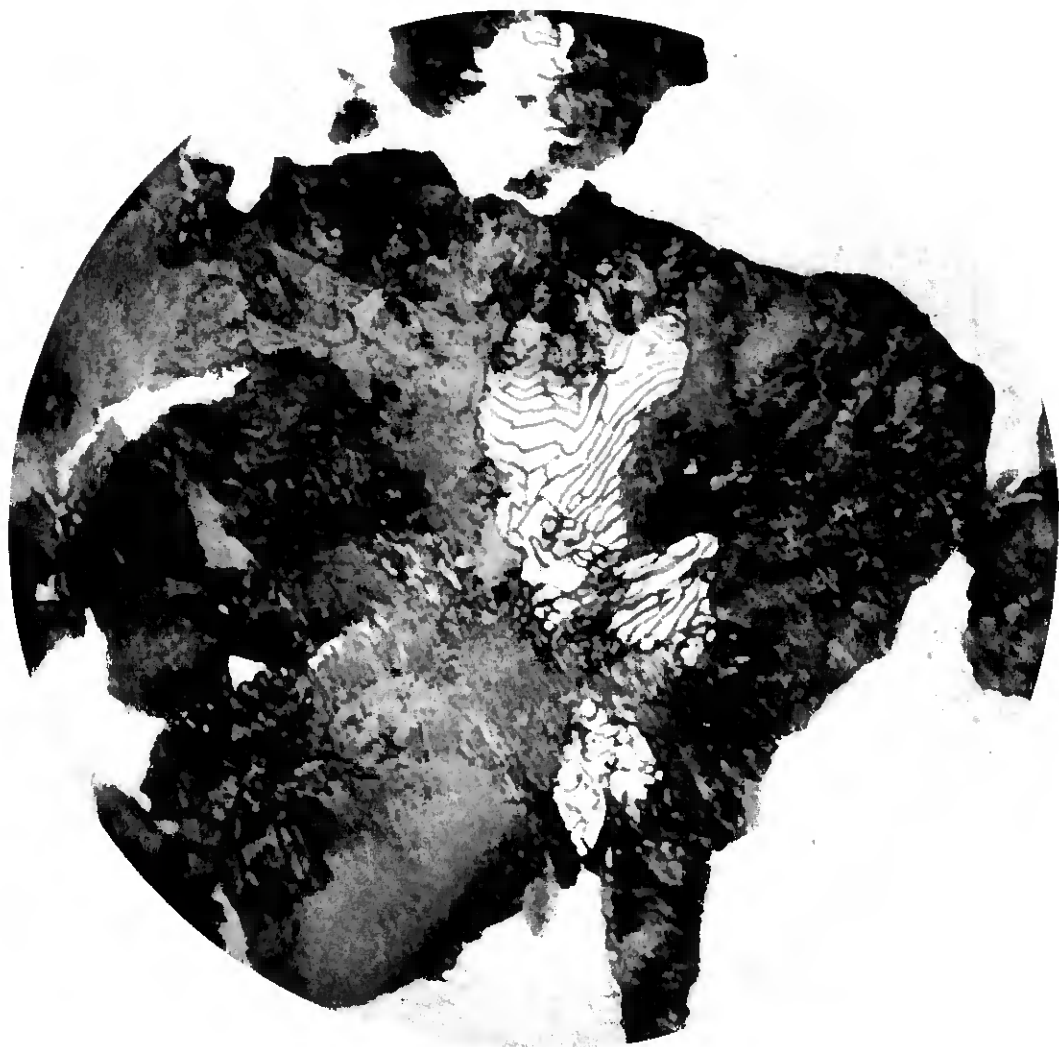
Fig. 11—Mag. 3500X. Fig. 11 illustrates the wide range in structure to be found in hardened steel. The background is martensite which contains a troostitic nodule. One grain of the nodule is fully laminated pearlite. The other grains are in all stages of stratification.
