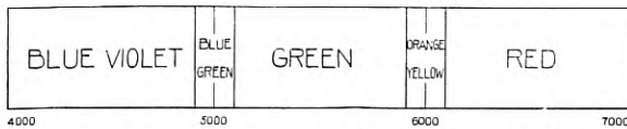
Fig. 8—Diagram representing the spectrum of arc light divided roughly into three dominant bands.
