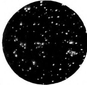
Fig. D. Colloidal particles as seen through the ultra-microscope. (a) Polymerized particles in a phenolic resin solution. Taken with the cardioid ultra-microscope and the Lucas Photomicrographic camera. Instantaneous exposure was necessary because the particles were in constant motion. Magnification, 220 X.
