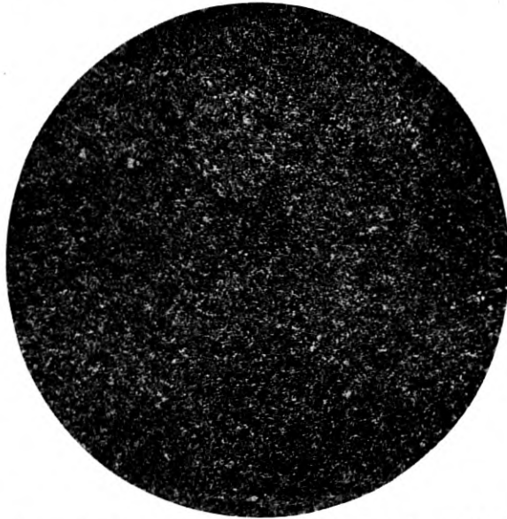
Fig. K. Steel of 1.5% carbon heated to 825° C. and quenched in oil. This medium-power photomicrograph at 100 X really tells very little about the steel, except that it possesses a fine structure.
