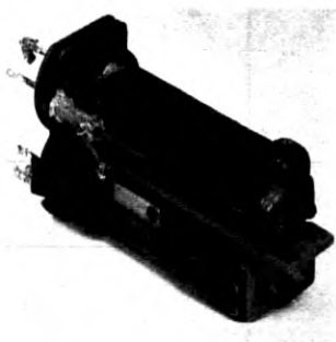
Fig. 9—Line and cutoff relays
