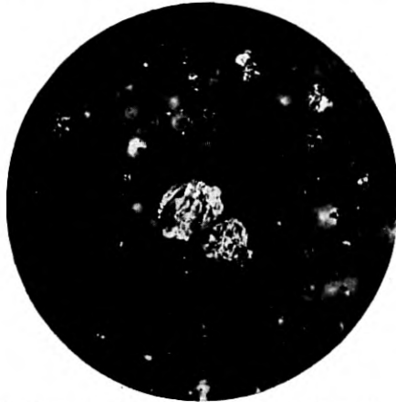
Fig. C. Distribution of filler particles in soft rubber insulation as revealed by a transparent section. The section was cut in a microtome by "flashing" the rubber with liquid air which hardened it just sufficiently to cut properly. The specimen was photographed by polarized light and with selenite plates to secure contrast between the particles and the embedding rubber compound. Note agglomeration of the particles into large masses. The ideal condition of distribution would be attained when each individual particle is surrounded by rubber. Magnification 720 X.
