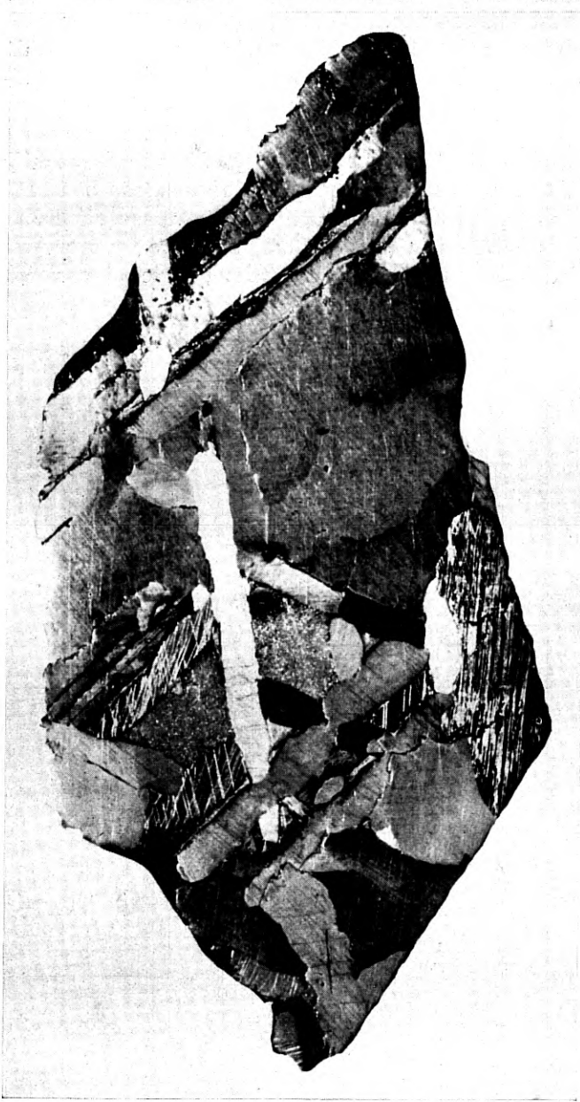
Fig. A. Meteoric iron consists of iron, nickel and the other elements usually found in steels such as carbon, sulphur, phosphorus, etc. The study of meteorites has contributed much valuable knowledge to the science of metallography. The Widmanstätten figures (shown by the arrangement of the constituents with reference to crystallographic planes) were generally considered characteristic of meteoric iron and it was believed that they were not to be found in manufactured iron and steel. Later this was shown to be an incorrect view.
