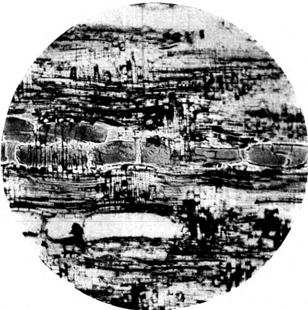
Fig. M. Direct color photomicrography by the autochrome process of a radial section of mahogany wood. Magnification 50 X. Mahogany is one of the best of cabinet woods and finds wide application in the telephone plant.
