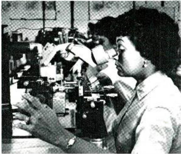
Operators use complex tools for thermo-compression bonding leads to transistor element stripes. Element is exactly positioned by micrometers.
