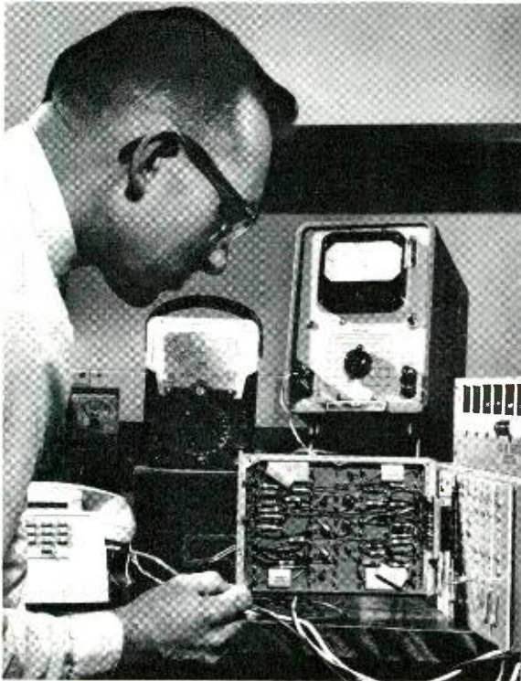
C. G. Morrison checks the circuit voltage on one of the plug-in units of a pushbutton receiver.
