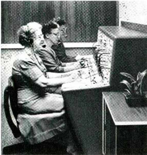
The 608A PBX switchboard is shown here in a three-position multiple arrangement. Each operator's position can be supplied as a single section.
