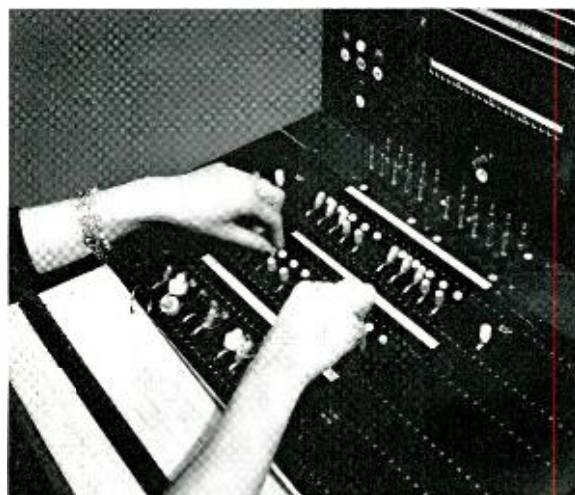
The controlled practice card (on left) indicates the various signals the control operator should send to the trainees. With this equipment she can simulate both "calling" and "called" parties.
