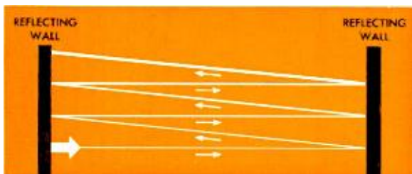
One arrangement of optical maser in which wave "grows" as it bounces back and forth between reflecting walls. (Vertical dimension of the diagram has been greatly exaggerated for clarity.)
