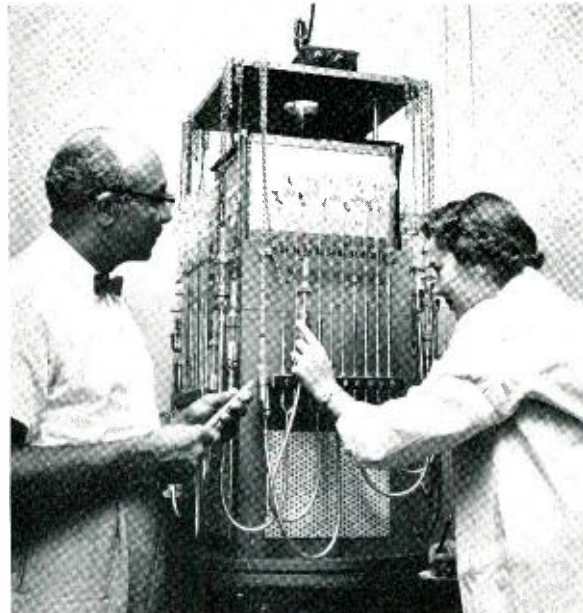
W. Lincoln Hawkins and Mrs. Mary Ann Worthington test effectiveness of recently developed thermal antioxidants used to protect polyethylene.
