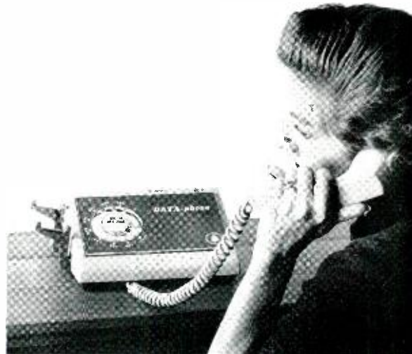
By dialing a number on a Data-Phone, this secretary can connect a machine—capable of sending hundreds of bits per second—to another machine.
