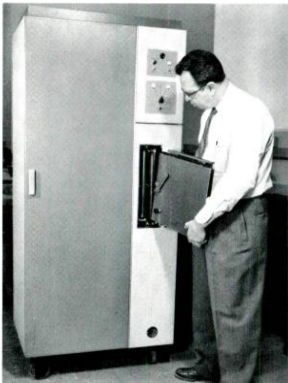
R. F. Glore attaching a cassette containing an exposed code plate to one of two loading stations of the trial Automatic Plate Processor (APP).
