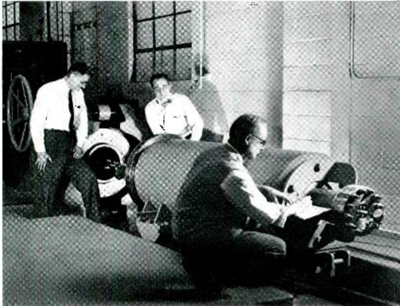
Engineers at the Hanover, N. J., Laboratory test ability of cable structures to withstand pressures even greater than those at ocean bottom.
