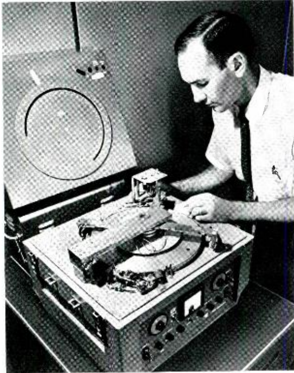
R. W. Lank adjusts the delay mechanism used to conduct simulated tests of satellite transmission.
