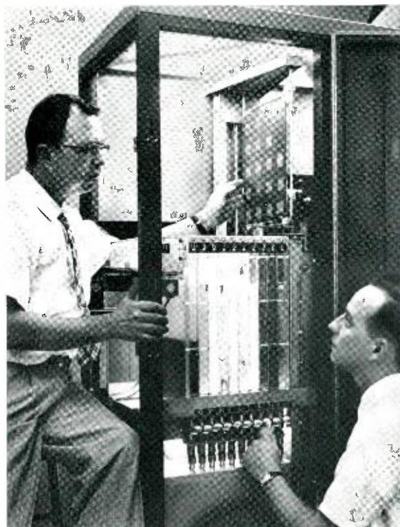
R. F. Glore, left, inspects encoding plate as R. K. Eisenhart adjusts chemical level in tanks. Color-coded solutions indicate mixture in each tank.
