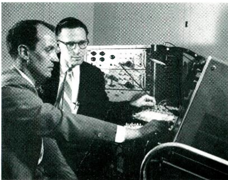
I. M. Ross, left, and L. A. D'Asaro examine with oscilloscope characteristics of the stepping transistor element in special circuit.
