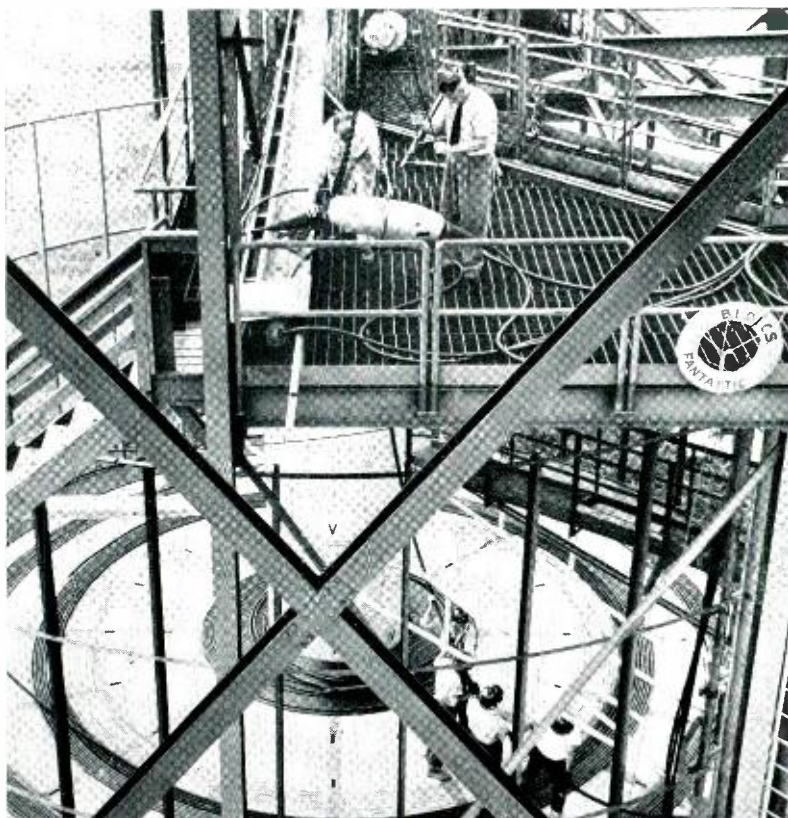
Two levels of the new "cable ship" show, on deck, engineers placing model of cable repeater in "highway" ready for launching, while below others work out methods of stowing coiled cable in "tank".
