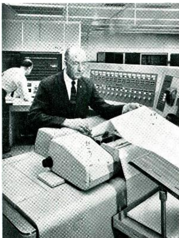
The author at the "in-process" printer of the 704 computer. This printer is used mainly to print instructions and intermediate results to guide the operator while a program is being run. In the background, G. H. Mealy is working at the switch panel of the main control center of the computer.
