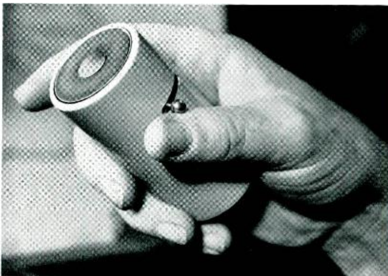
The new Bell Laboratories designed artificial larynx uses a modified telephone receiver unit to transmit sound through the user's throat.
