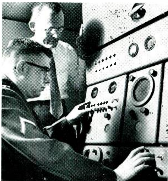
P. L. Hammann observes Army operator at the console of the missile tracking radar. Because much of the operation of this radar is programmed automatically, only one operator is needed here.
