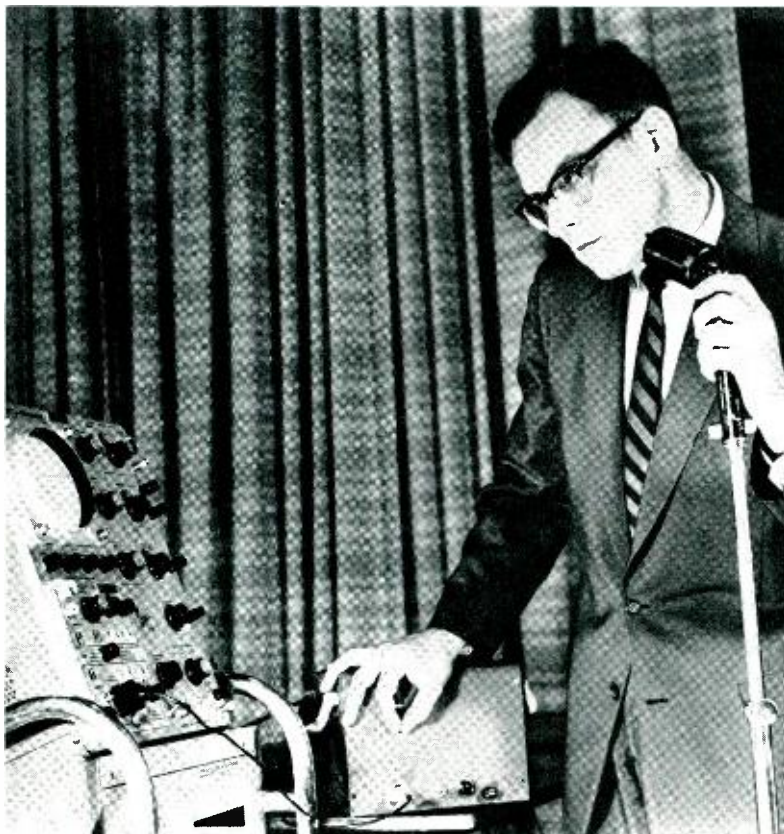
M. R. Schroeder switches on frequency-shift modulator, watches reverberations of his voice on oscilloscope. The reverberations shifted in frequency permit a two-fold increase in the loudness.
