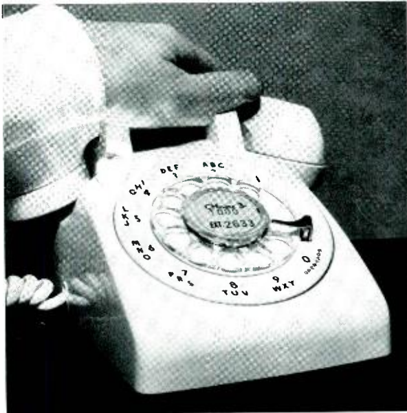
The new message-waiting telephone set. When a guest returns to his room and sees the lamp flashing on the room telephone, he calls the hotel or motel message center to receive his messages.
