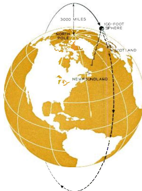
The geometry of a passive-reflector satellite in a polar orbit at an altitude of 3,000 miles, with terminals located in Newfoundland and Scotland.
