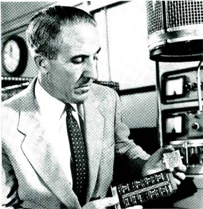
D. A. McLean compares reduced size of a printed circuit using the new sputtered thin-film resistors (in his left hand) with the comparable conventional printed-circuit board (in his right hand).
