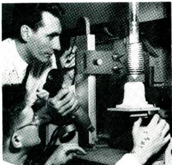
F. M. Smits (top) and R. L. Batdorf viewing the heated diffusion bucket inside the quartz envelope, which is circled by the RF induction coil.
