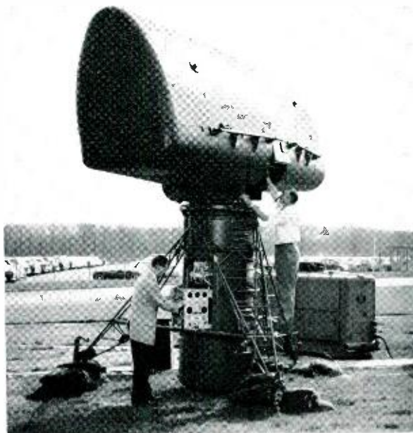
The author, left, examines transmitter panel of acquisition radar while C. E. Priefer checks inside glass fiber radome housing the antenna. This radar is controlled by operators in nearby van.
