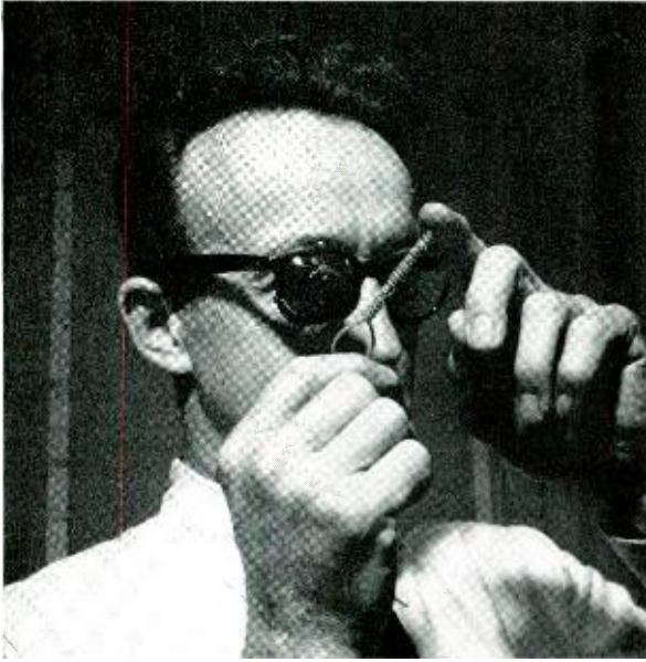
Author examines a wire coated with an unsatisfactory high-density hydrocarbon polymer that has been wrapped around itself. Exposure to elevated temperatures has embrittled the insulation so that it cracks at every convolution.
