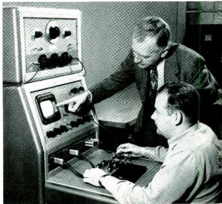
F. J. Hallenbeck, standing, explains the procedure for adjusting and final inspection. Inductor is adjusted until characteristic on oscilloscope matches trace of standard reference filter.
