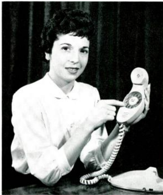
Mrs. Rose Calleo of Bell Laboratories demonstrates use of the new experimental handset. Dial near center of instrument protects against inadvertent operation and permits easy dialing.
