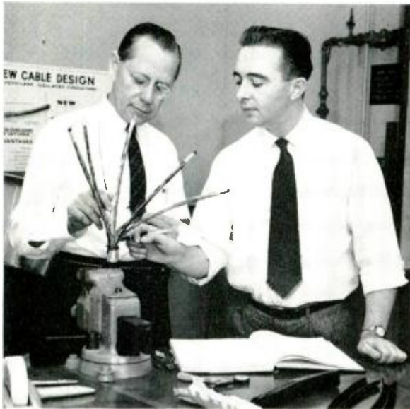
The author (left) and G. H. Webster examining arrangement of pairs in new even-count cable.
