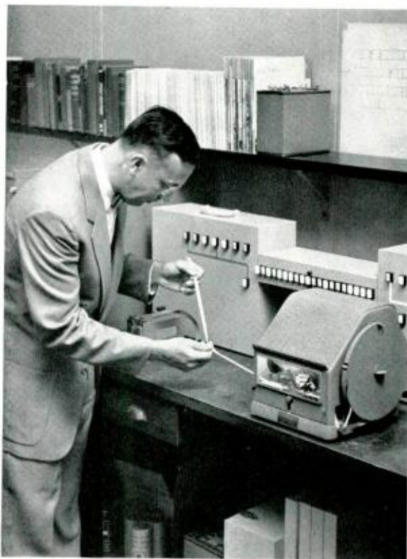
The author with the code-demonstrating device. Lamp displays demonstrate the code at any step in procedure of correcting errors in data signals.
