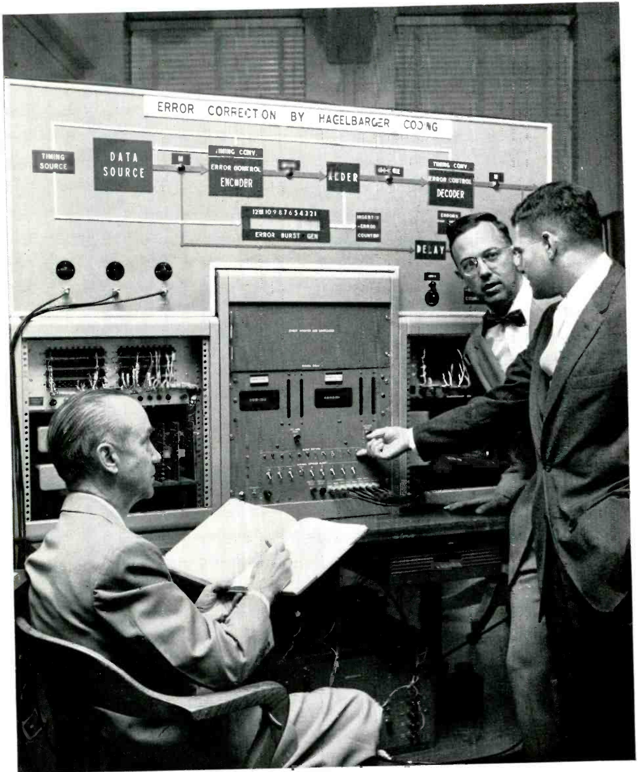
S. T. Meyer, left, D. W. Hagelbarger, and F. E. Froehlich discuss features of equipment which tests error correcting codes on actual telephone lines. Burst lengths and redundancies can vary.
