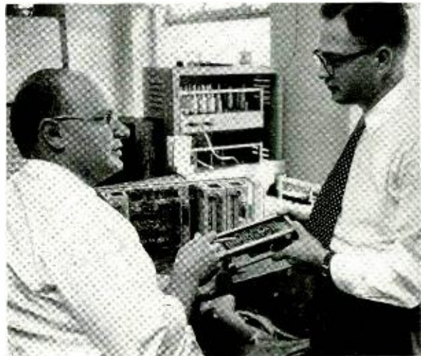
E. G. Spack (left) and the author inspecting circuit assembly used in the SAGE data signaling system. Communication over system is at the very fast rate of 1,300 or 1,600 bits per second.
