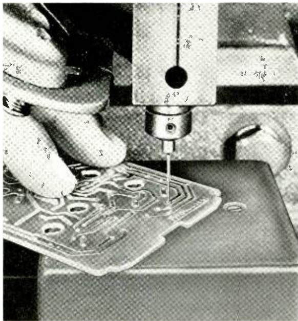
The eyelet-setting needle is shown in line with, and about to enter, the correct hole in a printed circuit board. The upper die is about to move downward to insert specific eyelet in the hole.
