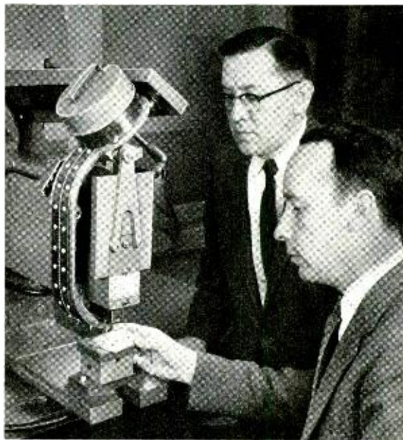
J. W. Buckelew (right) and E. D. Knab examine the new eyelet-setting machine. This over-all view provides an estimate of the machine size in relation to the circuit board and the operator.
