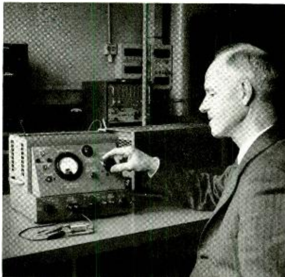
The author with a laboratory model of the new equipment for the surge-voltage testing of coils.
