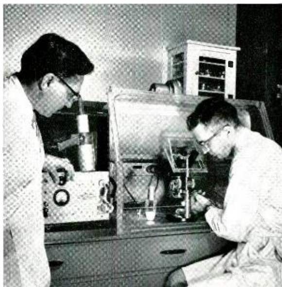
P. R. Pondy (left) and G. E. Helmke adjust air flow in assembly hood. Assembly operations are carried on inside carefully designed and controlled transparent hoods in special clean rooms.
