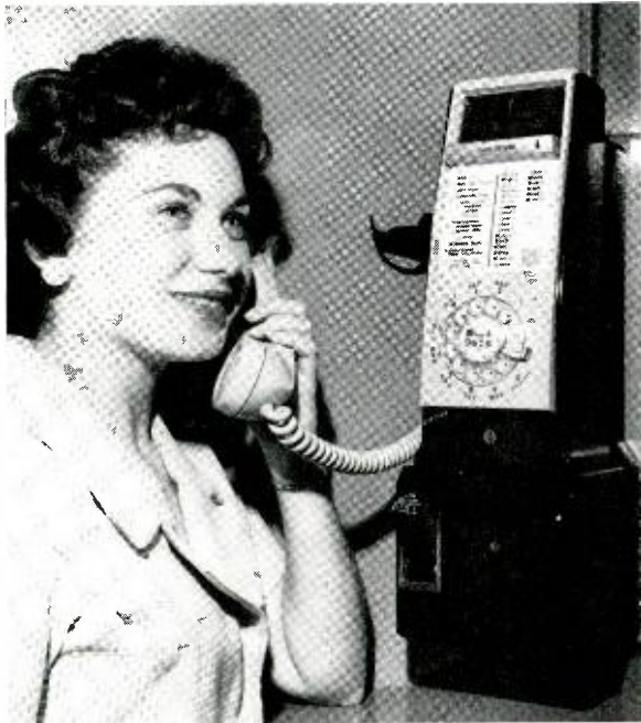
Mrs. Darleen Olsen of New Jersey Bell using the new coin telephone. "Edge-on" slot is at top of box.
