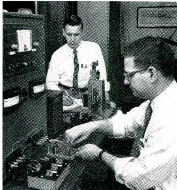
W. E. Asbell (left) and N. Wasserman making contact resistance measurements of connector.
