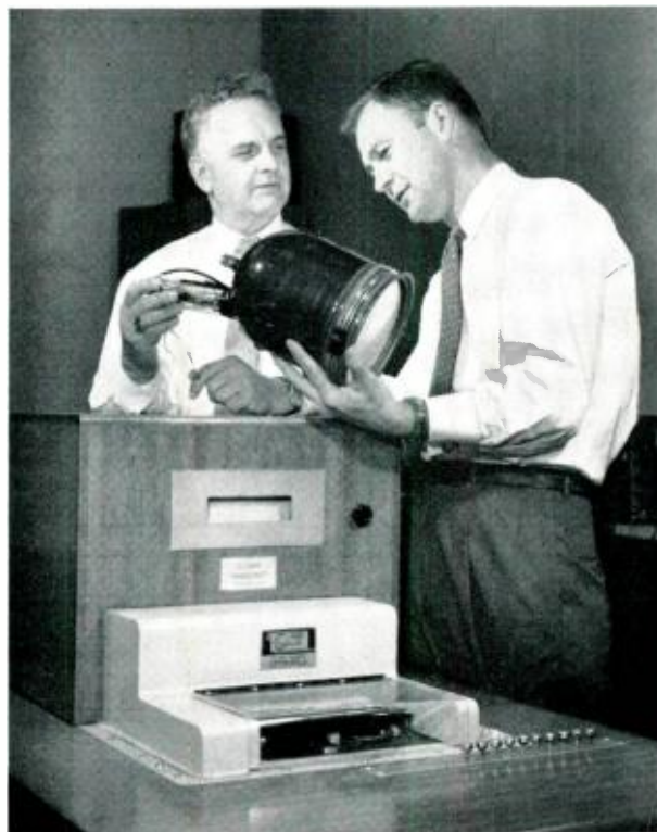
Fig. 6 — J. R. Hefele (left) and F. K. Becker inspecting direct-view storage tube used in signature-verification system for transmitting still pictures.
