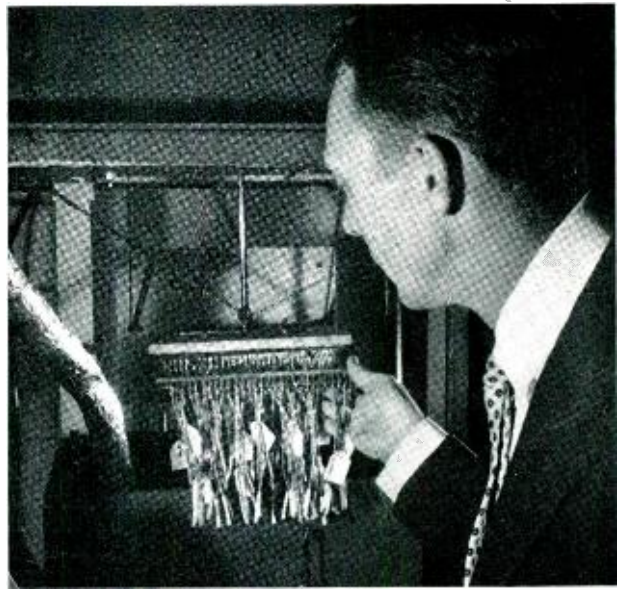
Fig. 3 — L. W. Faulkner loading racks of experimental cable-splice joints for automatic cycling.
