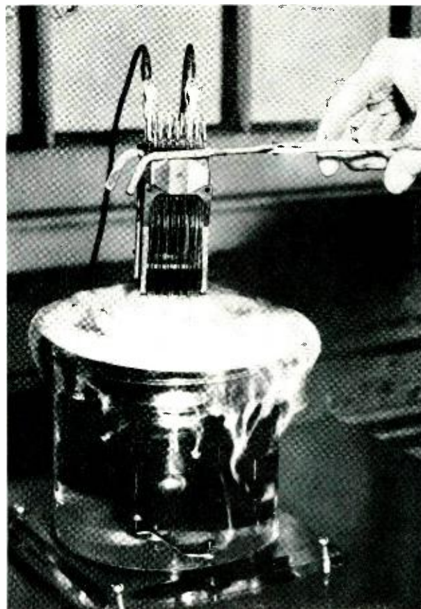
Fig. 4—Ultrasonic cleaning: steam is actually a mist of small droplets—the fountain effect—caused by ultrasonic agitation of trichlorethylene.
