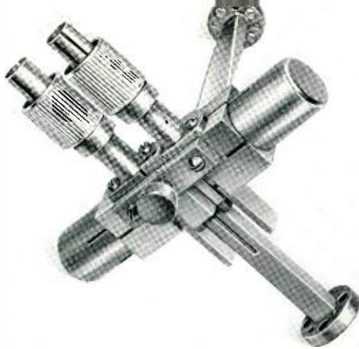
Fig. 5—Balanced mixer using two wafer-type rectifiers. This unit cancels noise sidebands.
