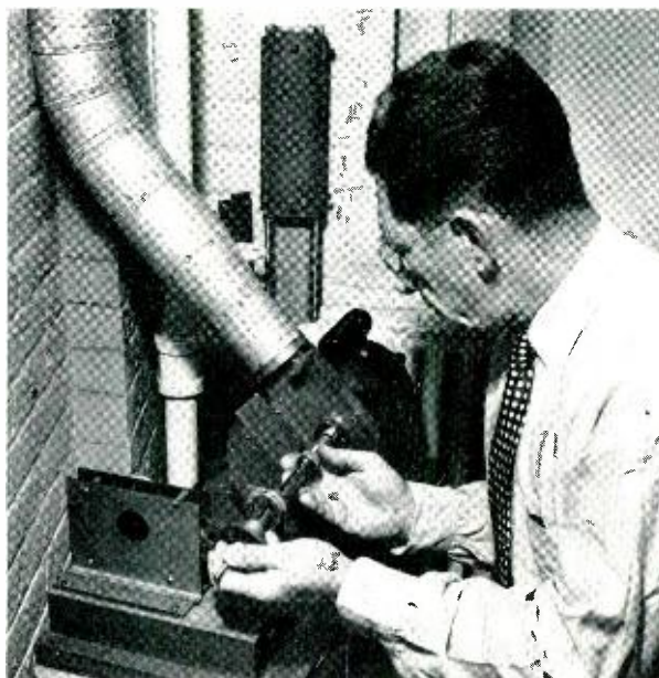
Fig. 2 — A. H. Yeager inserts a dust stick in generator for laboratory studies of contamination.
