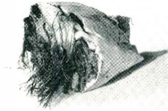
Fig. 2 — Barnacle removed from test rod wrapped with jute showing fibers cut and embedded in the calcareous base. Note sharp edges at rim of base. (Original magnification four diameters.)
