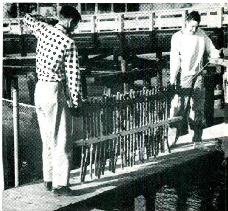
Fig. 6 — Member of Clapp Laboratories and L. R. Snook lowering a test rack into position at Wrightsville Beach.
