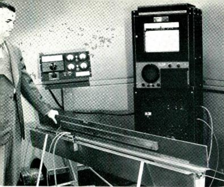
Fig. 2—Laboratory set-up including capacitance monitoring electrode (foreground), servo console, and operator's remote control panel (left background). S. C. Shores of the Laboratories demonstrates the use of the monitor in measuring the capacitance uniformity of an insulated wire.
