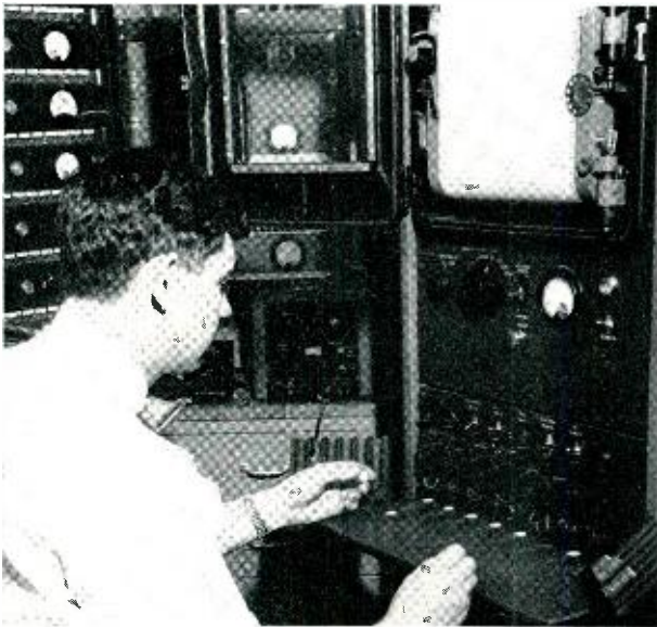
Fig. 1 — M. D. Patterson using test set for measuring varistors. Contactor has made connection to the sixth varistor from the left. Life-test rack can be seen in the background of the illustration.
