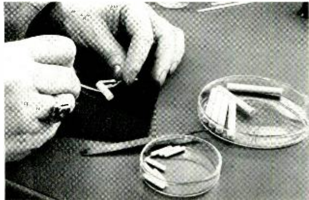
Fig. 2—Applying collodion to resistor core surface; two sizes of cores can be seen in foreground.
