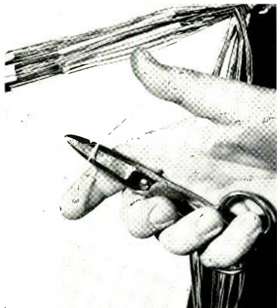
Notches in blade of scissors permit quick removal of plastic insulation.
