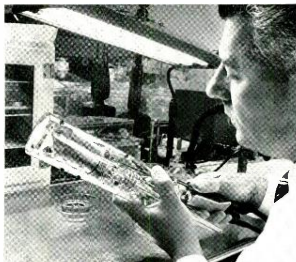
Fig. 4 — W. W. Baldwin welding leads to contacts on glass envelope of barrier-grid memory tube.
