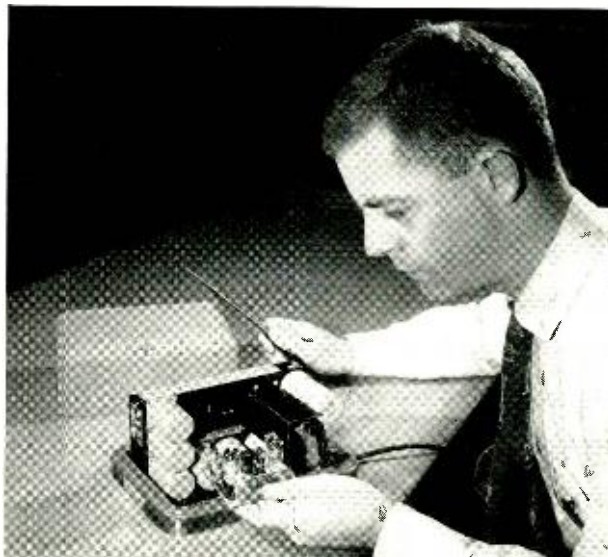
Fig. 1—W. J. Zinsmeister replaces an amplifier card in a Speakerphone box.
