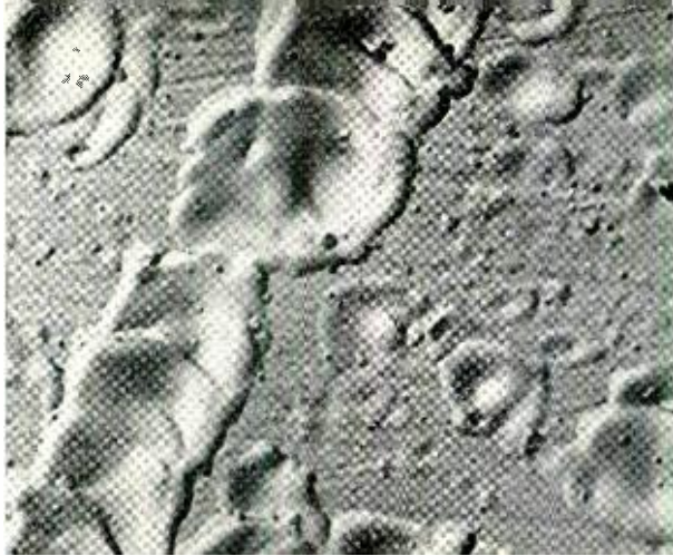
Fig. 4—Electron micrograph of a portion of the cathode mark due to a single “cathode” arc. Magnification 47,000 diameters.
