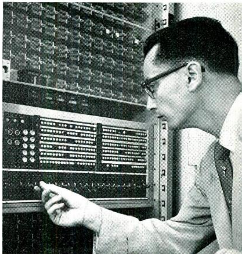
Fig. 6 — V. J. Acquaviva operates the test circuit control panel of the laboratory model.
