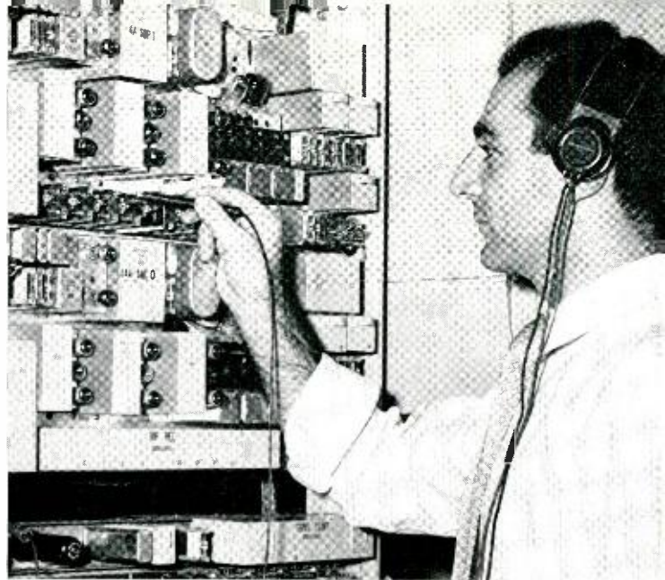
Fig. 1 — O. J. Russo tests a multifrequency receiver.
