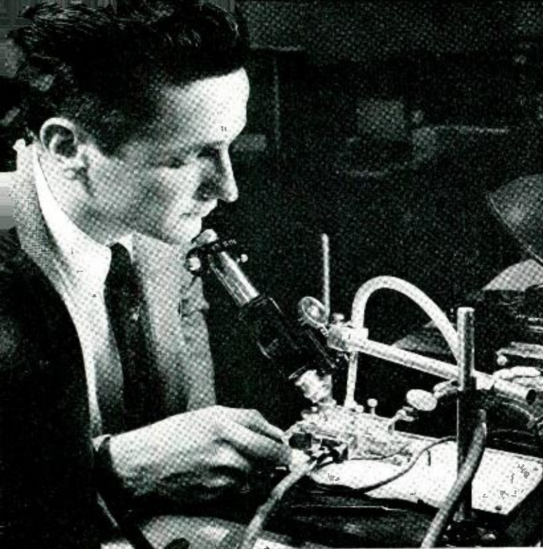
Fig. 4—W. L. Feldmann using micromanipulator to place gold and aluminum on silicon cube by alloying technique.
