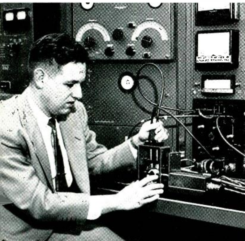
Fig. 6—W. L. Brune, who introduced the L3 transformer design into production, measuring the transmission characteristics of a completed unit.
