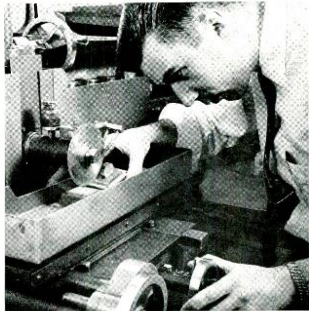
Fig. 3 — W. F. Flood placing section of ingot in position for sawing out germanium wafer.
