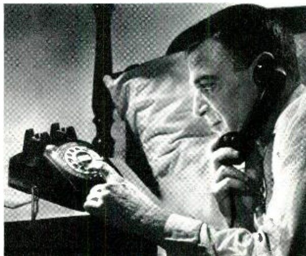
Dialing your bedside telephone in a darkened room is easy with this new 500-type set. When the handset is lifted, a small electric light comes on to illuminate the dial.
