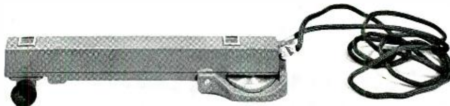
Fig. 2 — Range finder used for measuring wire clearances.
