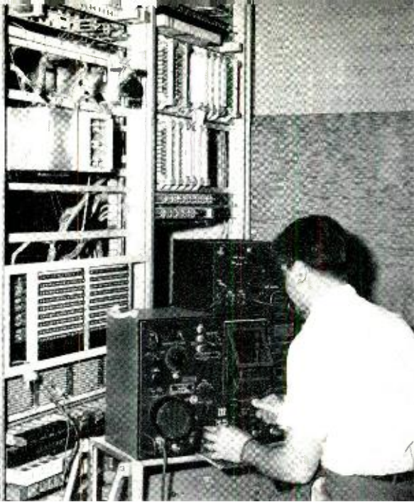
Fig. 1 — P. J. Cuffaro observing contact transient voltages by means of an oscilloscope. A camera is attached to this instrument to get photographs of the sort seen in Figure 7.
