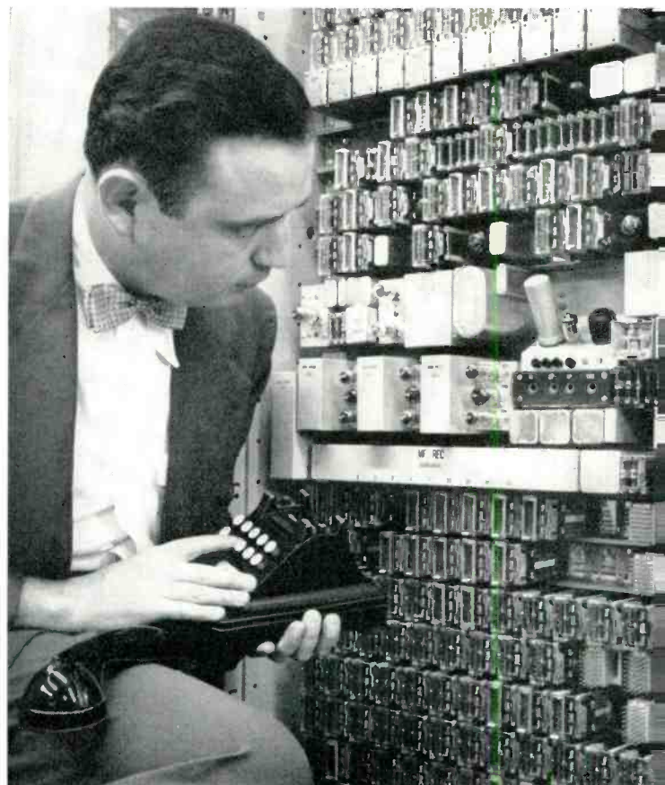
Fig. 2 — The author testing a new MF receiver with an experimental MF handset. The receiver is mounted in the Bell Laboratories wire spring No. 5 crossbar system.
