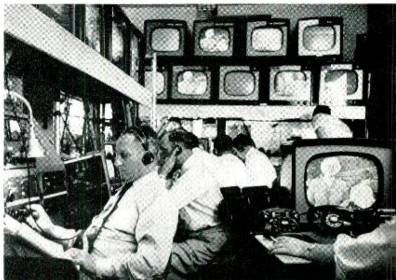
Control room for the closed-circuit TV loop shows pickups from several cameras on the monitors.
