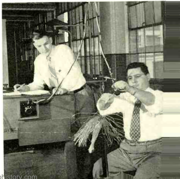
Fig. 2 — L. C. Graham and J. L. O'Toole testing aluminum conductor cable for capacitance in the Bell Laboratories laboratory at Kearny.
