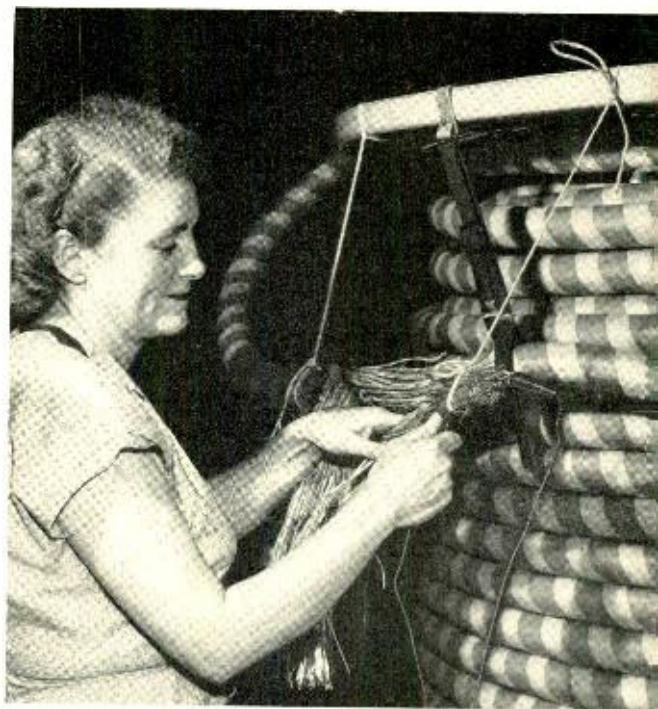
Fig. 3—Miss Mary Dempsey of Western Electric performing the "ring out" test for continuity of aluminum conductors in a cable prior to the sheathing operation.
