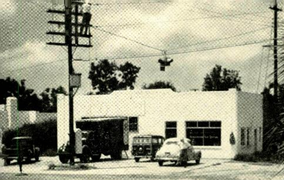
Fig. 2 — Outside view of the Hamokahodo test station. The pole in front of the station carries a pair of conductors from which noise was recorded during some of the thunderstorm periods.
