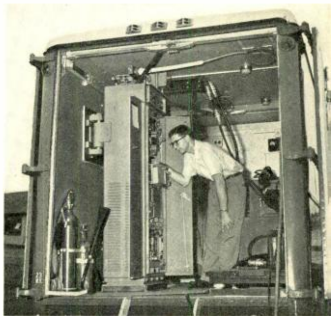
Fig. 2 — The pulse transmitter mounted in the truck is inspected by J. A. Smith.
