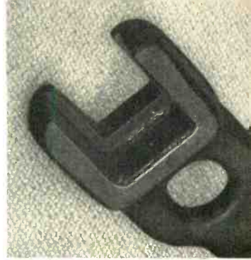
Fig. 2—One end of the wrench showing two sizes of openings and the elliptical hole.
