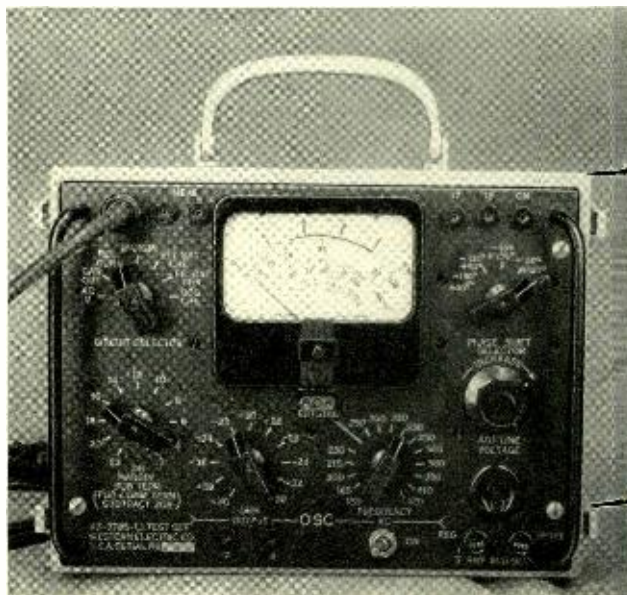
Fig. 1—The KS-5785 test set designed for maintaining M1 carrier terminals.
