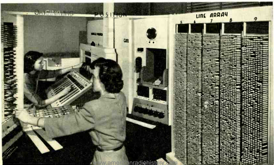
Fig. 1—A machine to simulate functions of a cross bar system. Pegs at right represent subscribers. Selected by random sampling, a peg is removed, attached to a report card, then routed through the various positions. At each, a girl records details for subsequent analysis.
