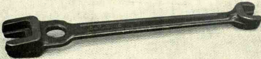
Fig. 2—One end of the wrench showing two sizes of openings and the elliptical hole.
