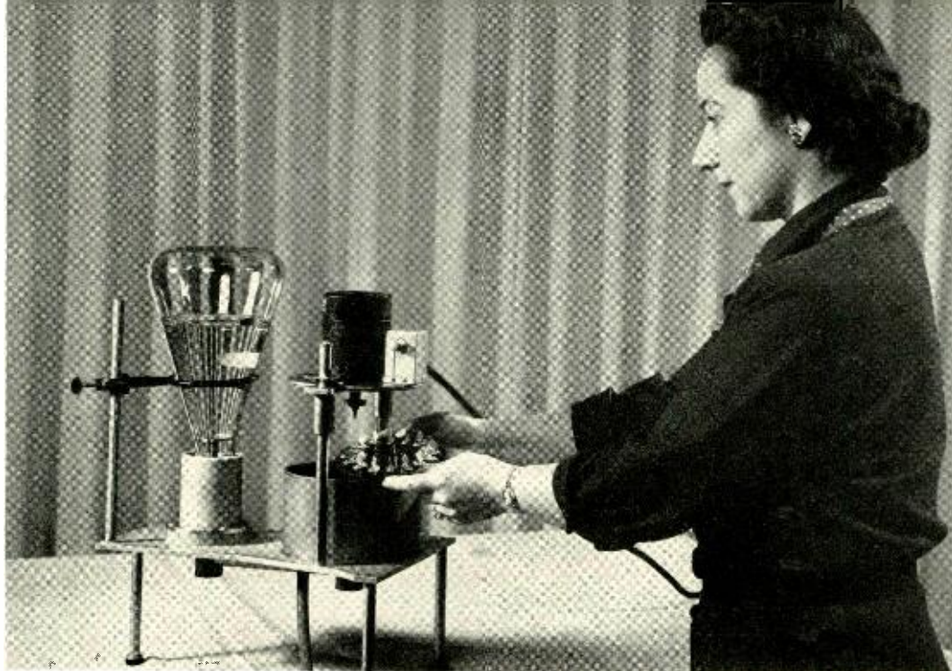
Fig. 1—Dorothy Schmidt loads the degreaser with quartz crystal units. Trichloroethylene from the reservoir at left is vaporized when pumped under a force of 100 lbs. per square inch as a spray against the wall of the cleaning compartment (not shown). The vapor collects on the crystal units in droplets which clean as they flow over the surface.
