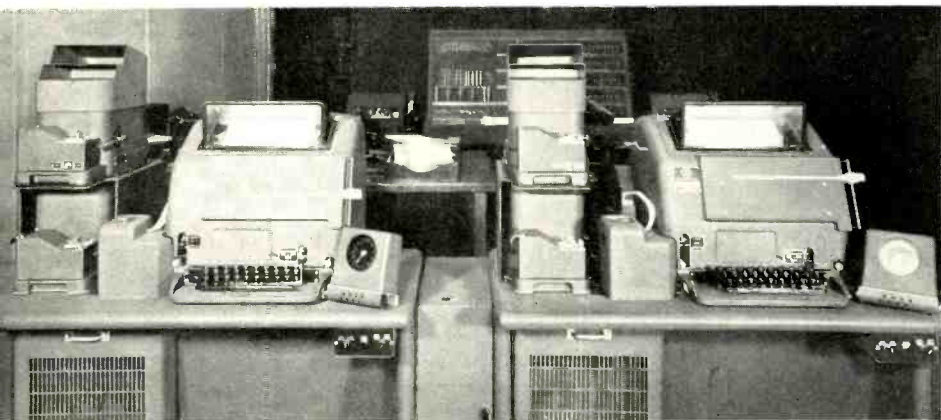
Fig. 4—Local outlet machines: two teletypewriters and one typing reperforator for receiving messages at the switching office. As will be noted, considerable attention was paid to appearance.
