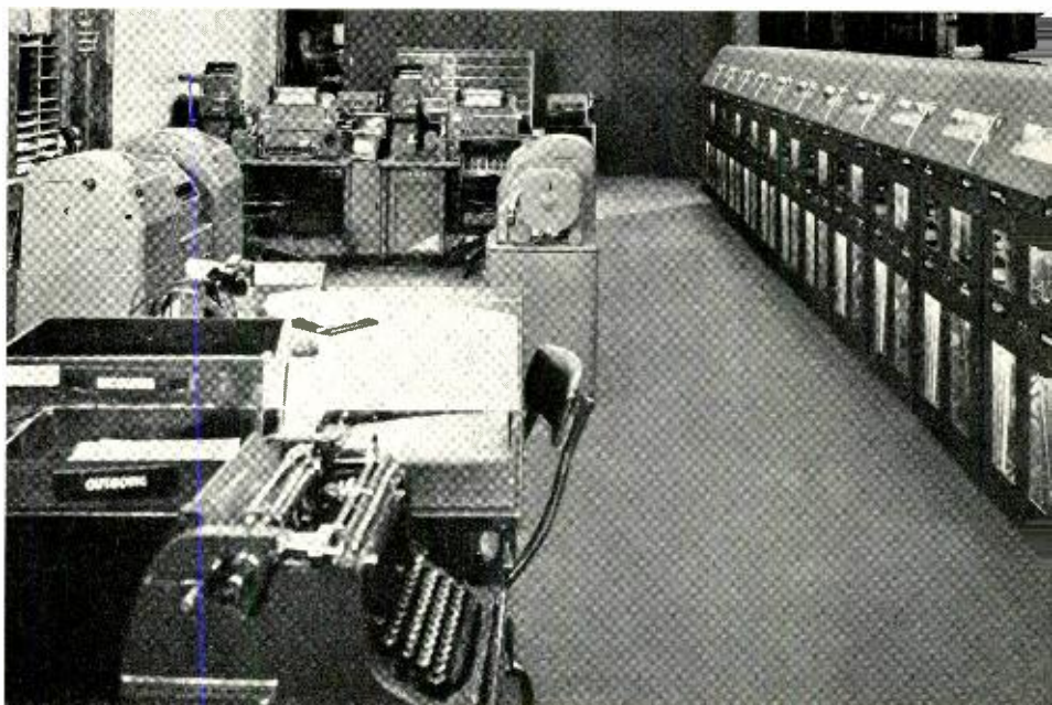
Fig. 1—General view of the operating room of the Pan American Airways installation. Reperforator transmitter cabinets at the right and one line of relay cabinets in the background.
