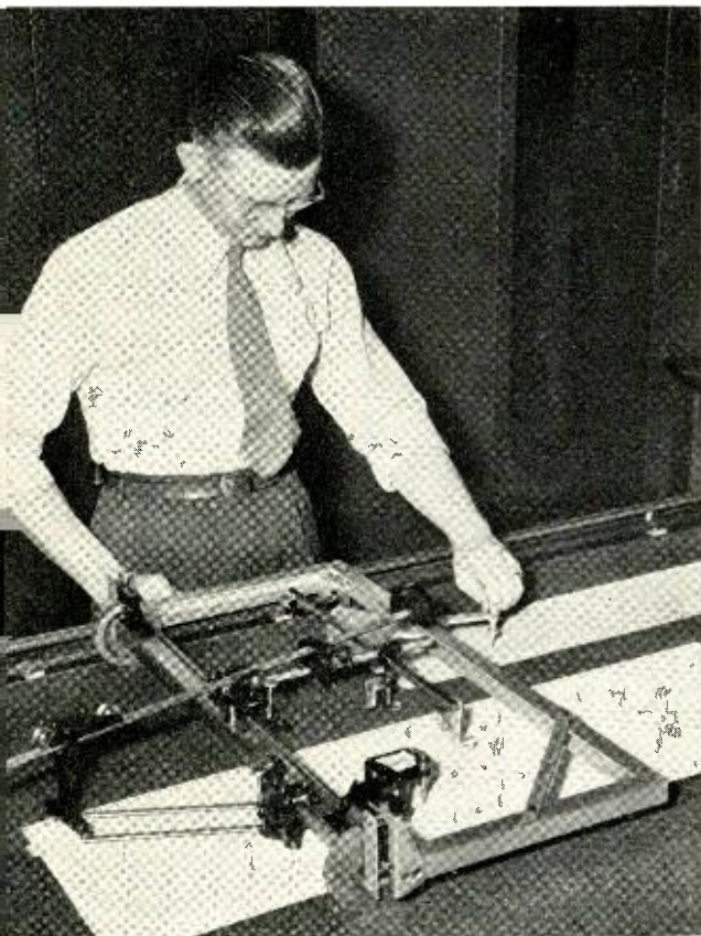
R. W. Marshall operating the modified Coradi integragraph to determine phase distortion.
