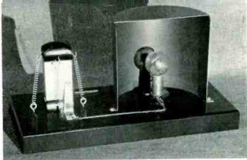
Fig. 3—The first lecture aid to be built was for demonstrating the piezoelectric effect. At the left is a large block of piezoelectric crystal which when struck with a small gavel generates a voltage that lights the lamp at the right
