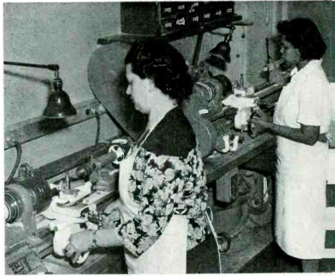
Fig. 2—Some ceramic parts are made on a lathe. They must be oversize, to allow for shrinkage during firing
