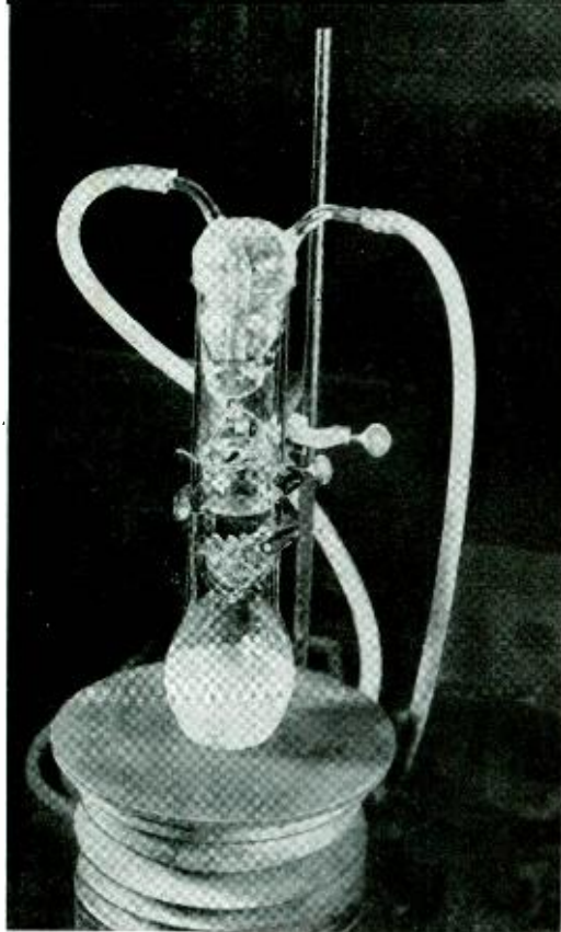
Fig. 2—Synthetic rubber copolymer was separated from other ingredients by extracting it with a constant boiling mixture of toluene and ethyl alcohol
