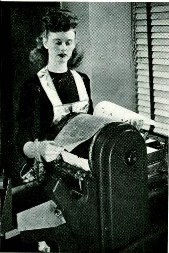
Some 26,000 sheets of mimeograph and hectograph reproductions are turned out daily at West Street, where peaks as high as 185,000 sheets a week have been reached. Here, Alice Bugler, one of ten girls engaged in this work, puts a stencil on the cylinder of her mimeograph machine preparatory to running her assignment
