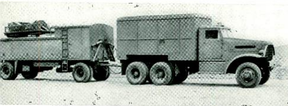
Fig. 2—Power truck and trailer of the SCR-545-A radar folded for travel
