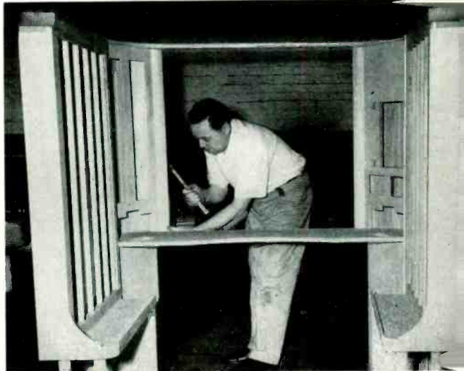
Below: Cabinetmaker H. H. Carlisch completes a synthetic traffic study machine for the No. 5 crossbar
