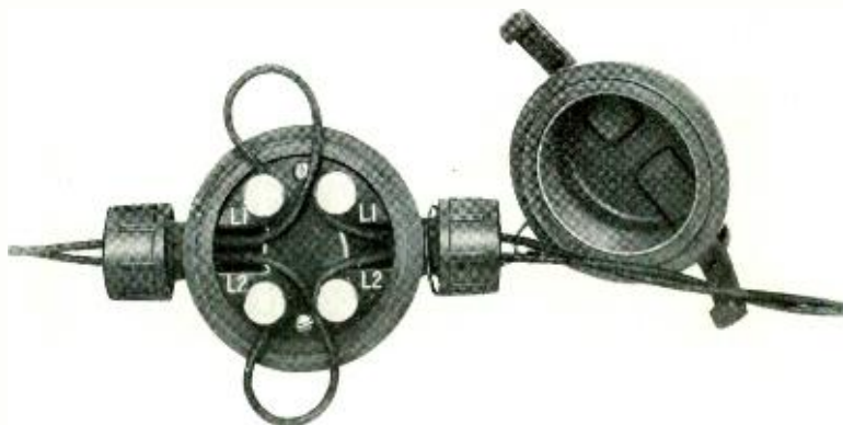
A loading unit with cover removed showing method of fastening wires
