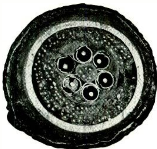
Six-unit 0.27-inch coaxial used between Atlanta, Ga., and Meridian, Miss.
