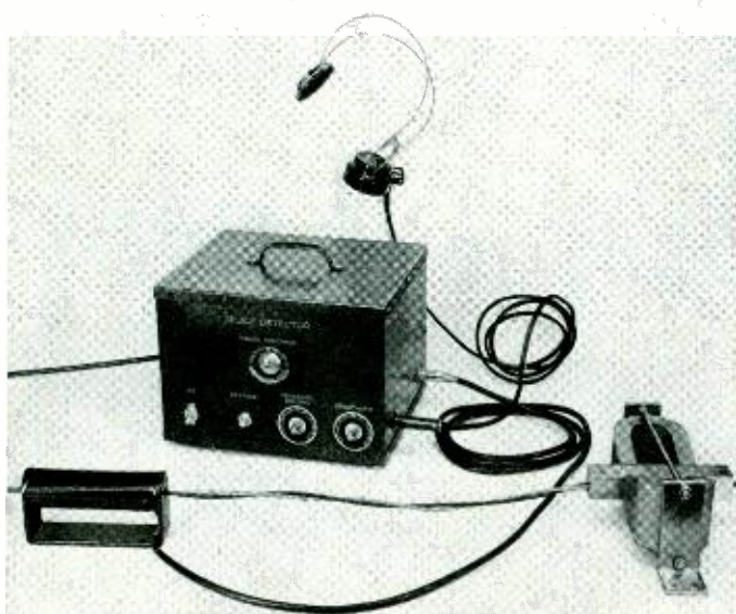
Fig. 1—To detect splices, wire is passed through the magnetizer at the right, and then through the detecting coil at the left. The presence of a splice is evident on the visual indicator of the splice detector
