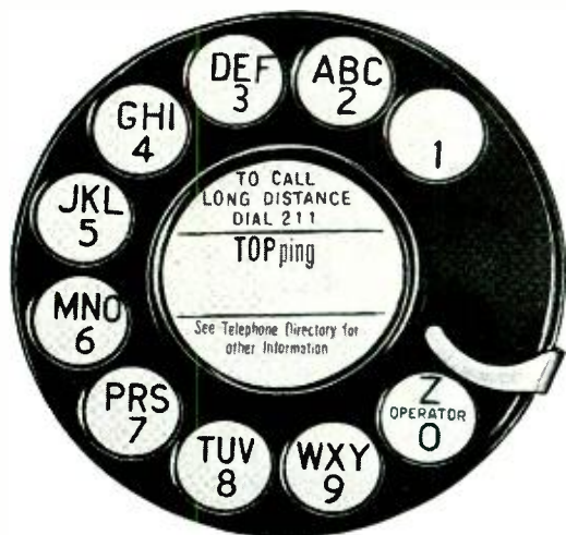
Fig. 1—The telephone dial has letters in only eight of the ten finger holes
