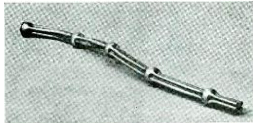
Fig. 2—Section of a coaxial conductor used as an antenna feed line that was completely collapsed by lightning current flowing along it
