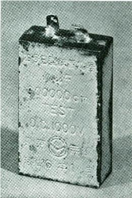
Japanese capacitor taken from a captured field telephone set
