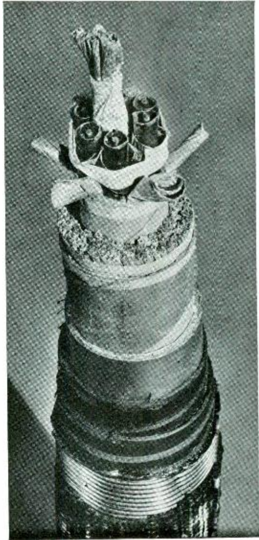
Fig. 4—The new lightning-protected cable
