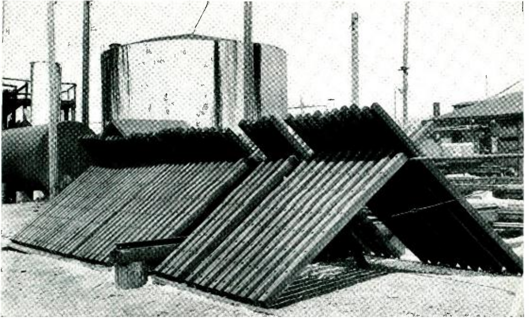
Fig. 4—Testing crossarms for tendency to bleed, check, twist and warp by X-piling on a rail
