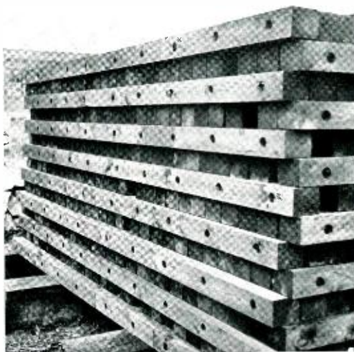
Fig. 3—In a new method of stacking cross-arms for curing, the overlapping of the alternate tiers protects their ends and prevents warping and twisting during drying
