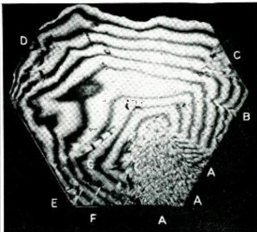
Fig. 9—The same crystal as Figure 8, but turned to bring the optical axis parallel to the line of sight. Note greater width and separation of contour bands
