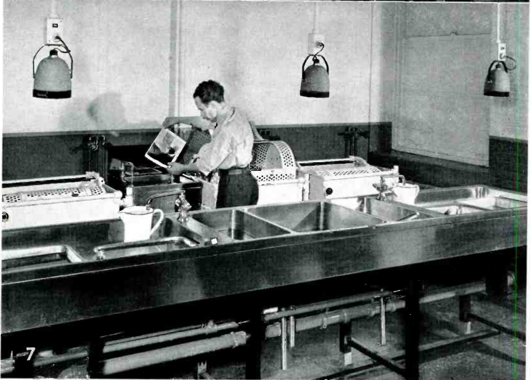
Figs. 5, 6 and 7—One of the two printing machines, operated by G. T. Scheeler, is shown in Figure 5. A similar machine is to the right of it, separated by a table. On the opposite or east wall, and separated from the printers by the long developing tanks, are the rotary washers, shown in Figure 7 with F. Fossetta. The developing room includes along the north wall a two-compartment developing tank, shown with S. O. Jorgensen in Figure 6. On the south wall are work benches and on the west wall is the film drier which may also be reached from the finishing room
