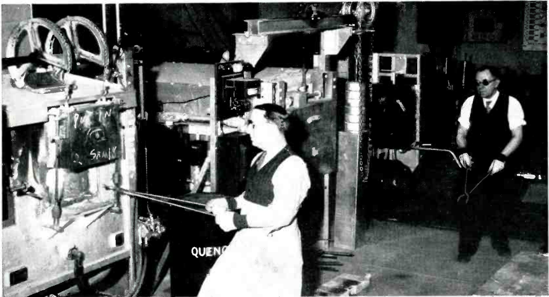
The metallurgical laboratory at Murray Hill is well equipped with electrically heated furnaces and rolling mills for use in studying the properties of metals and alloys. R. J. Reilly is about to remove a heated billet from one of the furnaces. M. Tompa is the second mill operator
