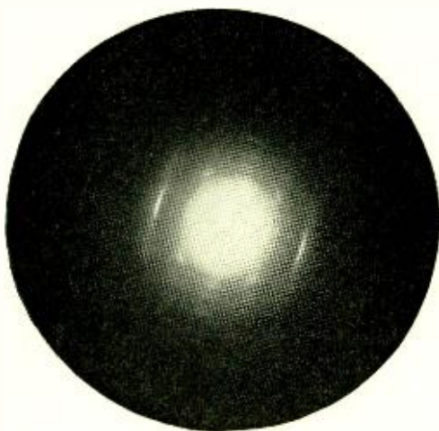
Fig. 3—The electron-diffraction pattern of gutta-percha, a source of information about the structure of this complicated molecule
