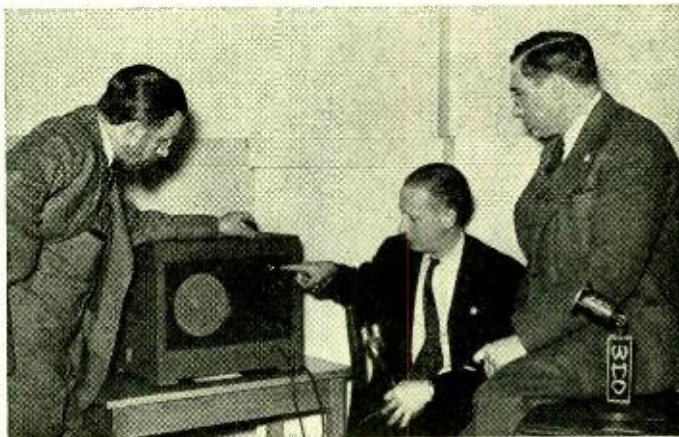
The Mirrophone, developed for the Western Electric Company by the Laboratories, already has a number of diverse applications to its credit. One midwestern radio station, for instance, has a Mirrophone set up in its announcers' room. As each announcer comes on duty, he reads his commercial copy to the Mirrophone, then listens to the playback. Station executives say that the announcers, able to hear and criticize their own speech without the delay attendant on processing "wax" recordings, have greatly improved their work. One of the radio stations which uses the Mirrophone is WHO, Des Moines, Iowa. Shown above are, left to right: Colonel B. J. Palmer, President, Central Broadcasting Company, which owns and operates WHO; Bobby Griffin, veteran WHO announcer; and Harold Fair, WHO's Program Director
