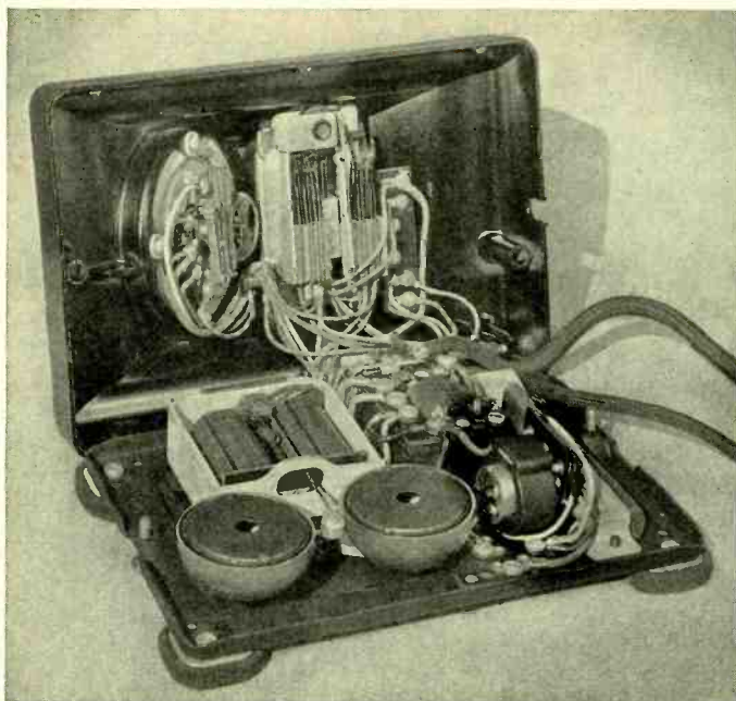
Fig. 1—In the new subset, the amplifier occupies a space less than one of the bells
