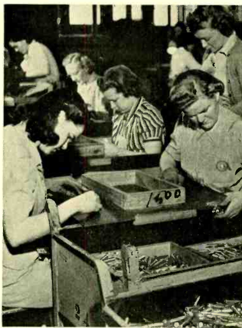
Educated fingers and trained eyes pass the perfect cartridges into trays and reject those with scratches and other surface imperfections. Every cartridge is given this hand-visual inspection
