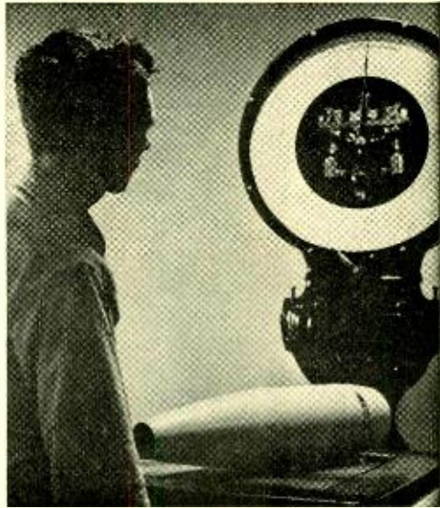
Weighing in for the big battle, loaded shells step on the scales just like the fighters they are. The operator classifies this 155-mm shell to determine range table
