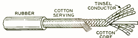
Fig. 3—The new rubber-insulated conductor for switchboard cords has a serving of cotton over the tinsel conductor and a thin outside layer of rubber applied by a continuous vulcanizing process
