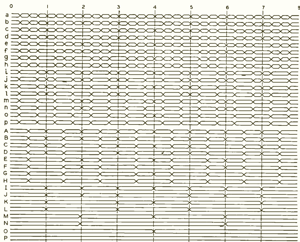
Fig. 2—Fundamental types of transpositions requiring 31 transposition poles
