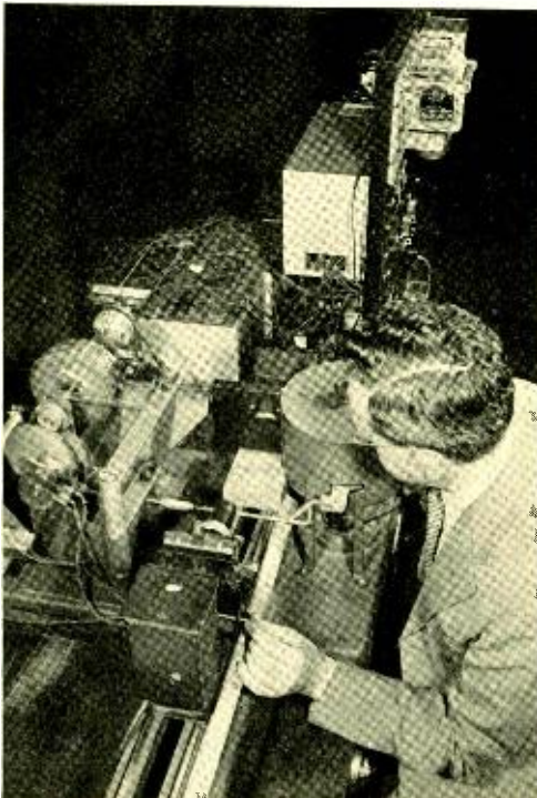
Fig. 1—Optical curve analyzer which can measure the first thirty harmonics of a complex sound in a minute and a half
