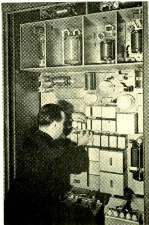
Fig. 4—On the rear of the transmitter are the coils, condensers, and the voltage regulator, evident at the right
