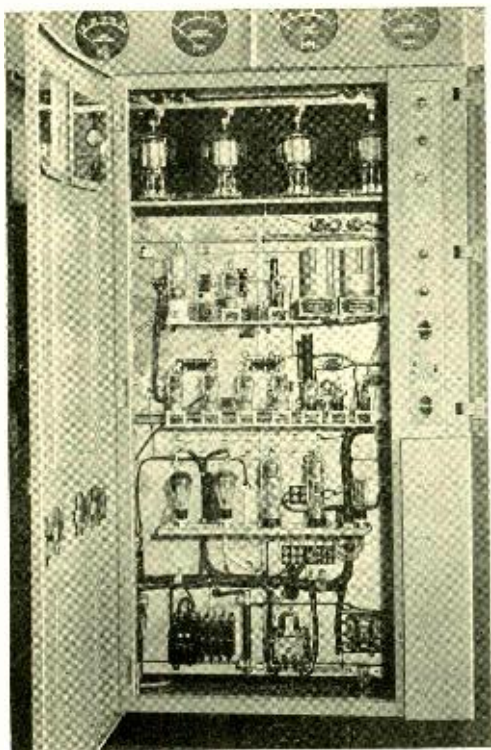
Fig. 3—Front view of 443-A-1 radio transmitter with door open
