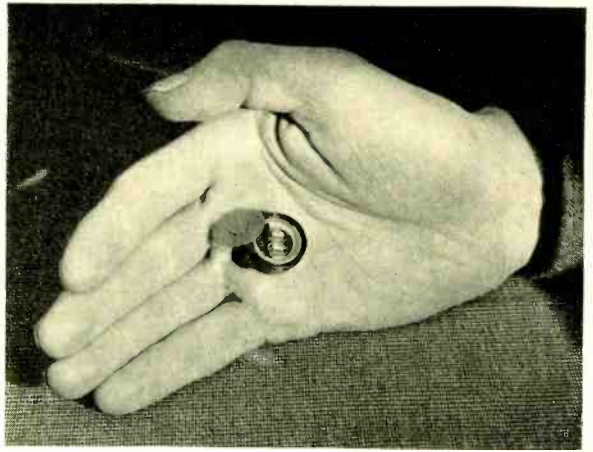
Fig. 4—Receiver unit for the new audiphone showing permalloy disc on diaphragm
