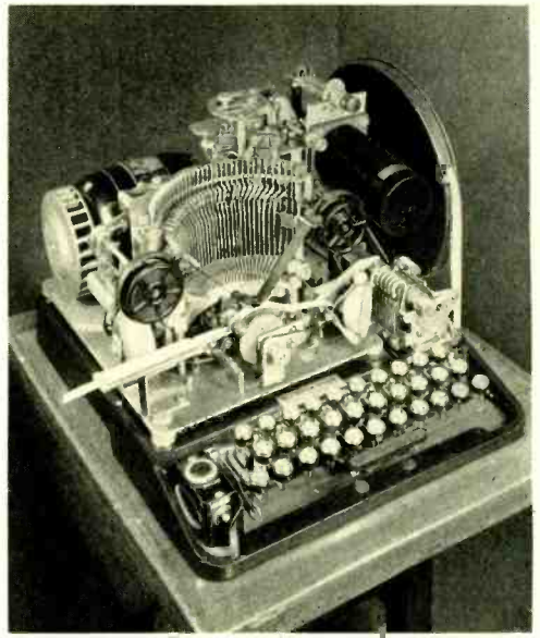
Fig. 5—No. 14 standard tape teletypewriter of the Bell System (cover removed). It is type-bar operated and uses an inking ribbon
