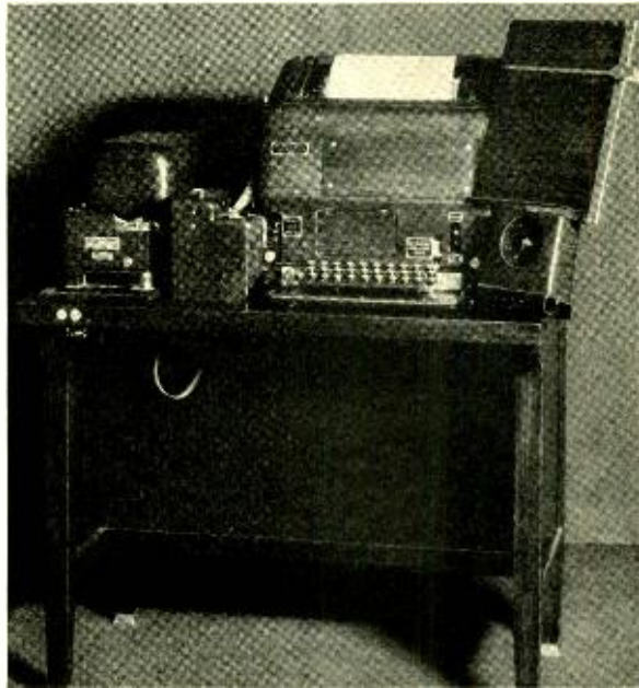
Fig. 6—No. 19 page-printing teletypewriter set arranged for tape transmission. The message can be typed on paper and punched in a tape simultaneously
