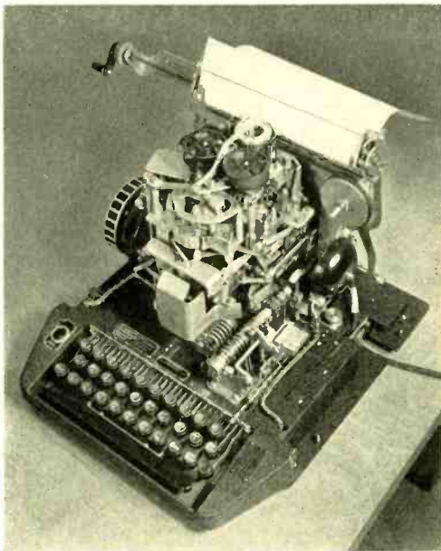
Fig. 4—No. 26 teletypewriter (cover removed) designed for service where only an original or at most one or two carbon copies are required. It has a movable carriage and the type characters are mounted on a wheel
