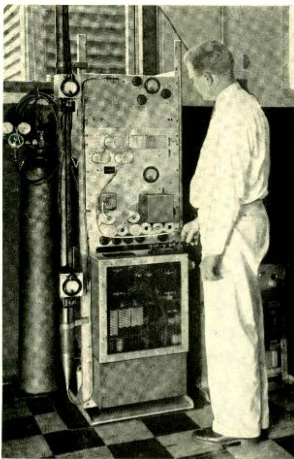
Fig. 1—Transmitting equipment for making fading tests at Lawrenceville, New Jersey
