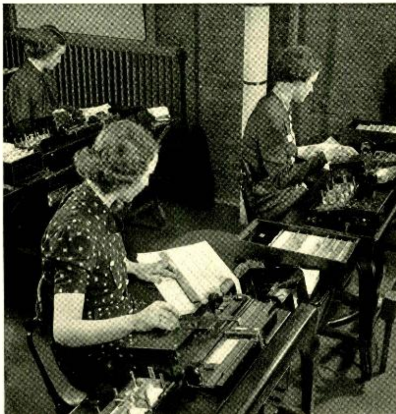
Laboratories expenditures are recorded and summarized by these Hollerith Key Punch Machines. The original data are transcribed on tabulating cards in the form of punched holes
